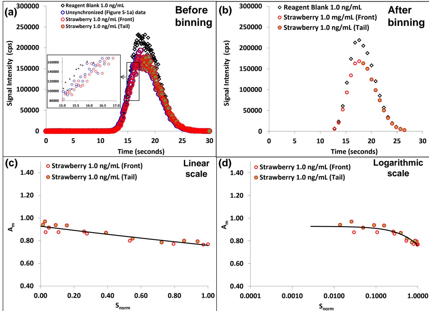
**Figure S-2.** Calculation of  $A_m$  as a function of  $S_{norm}$  for hexazinone in strawberry extract from synchronized data. Averaged MS/MS chromatograms: (a) all data points and (b) binned. The strawberry data shown on panel (a) has been shifted by +120 milliseconds (see inset). The resulting  $A_m$  vs.  $S_{norm}$  graphs are shown in (c) linear and (d) logarithmic abscissa scales.
