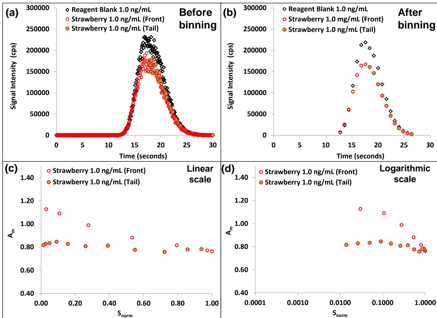
**Figure S-1.** Calculation of  $A_m$  as a function of  $S_{norm}$  for hexazinone in strawberry extract from unsynchronized data. Averaged MS/MS chromatograms: (a) all data points and (b) binned. The resulting  $A_m$  vs.  $S_{norm}$  graphs are shown in (c) linear and (d) logarithmic abscissa scales.
