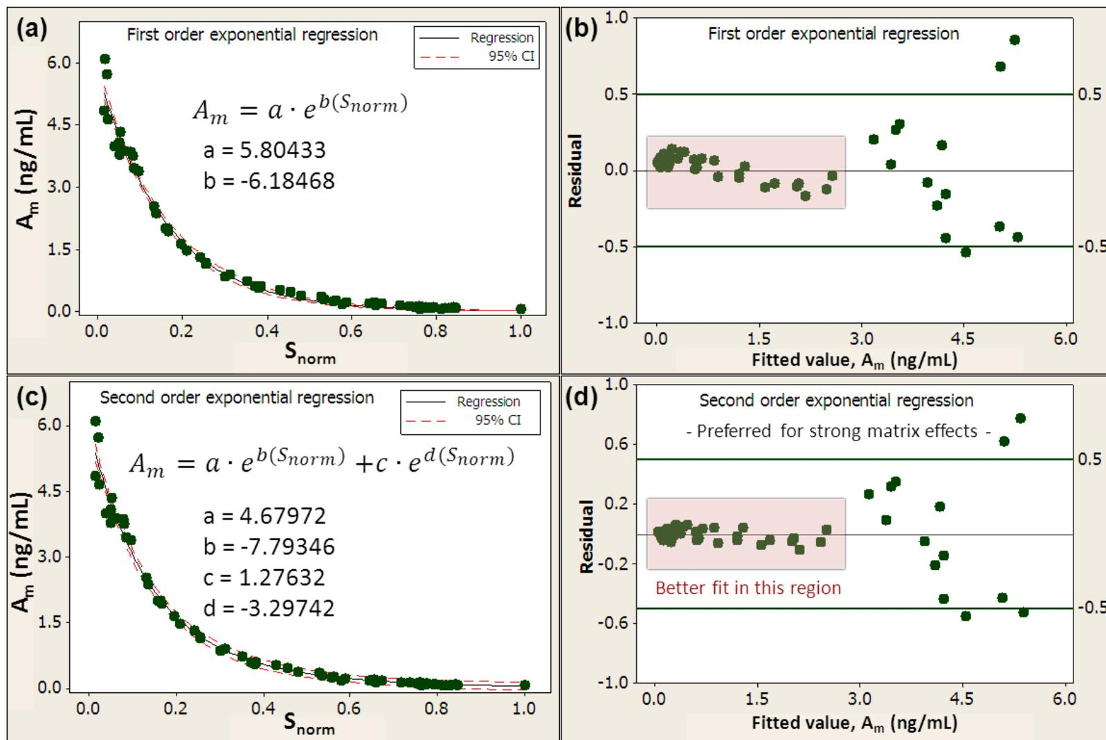
**Figure S-5.** Non-linear regression results obtained for hexazinone in canola seed at 5.0 ng/mL. Top panels: (a) first order exponential regression and (b) corresponding residuals. Bottom panels: (c) second order exponential regression and (d) corresponding residuals. The residual plots have been scaled to the acceptable range,  $\pm 20\%$  of  $A$ , with reference lines at  $\pm 10\%$  of  $A$ .
