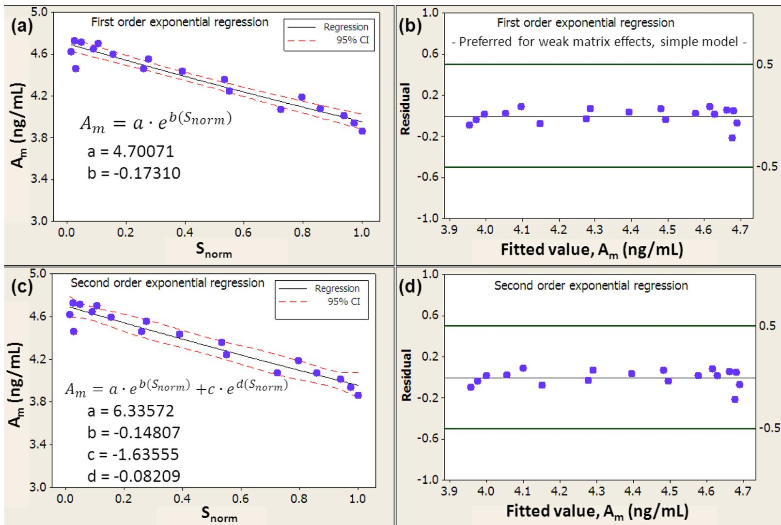
**Figure S-4.** Non-linear regression results obtained for hexazinone in corn meal extract at 5.0 ng/mL. Top panels: (a) first order exponential regression and (b) corresponding residuals. Bottom panels: (c) second order exponential regression and (d) corresponding residuals. The residual plots have been scaled to the acceptable range,  $\pm 20\%$  of  $A$ , with reference lines at  $\pm 10\%$  of  $A$ .
