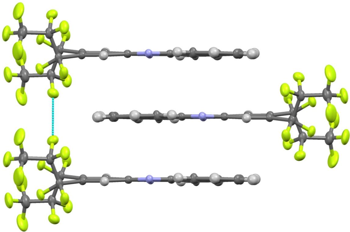
Figure S29: F-F short contact ( $C_{sp^3}$ -F-F- $C_{sp^3}$  attractive intermolecular interactions) observed between alternative molecules of **3** in crystal packing: (color code: light green, F; light blue, N; gray, C; white, H).
