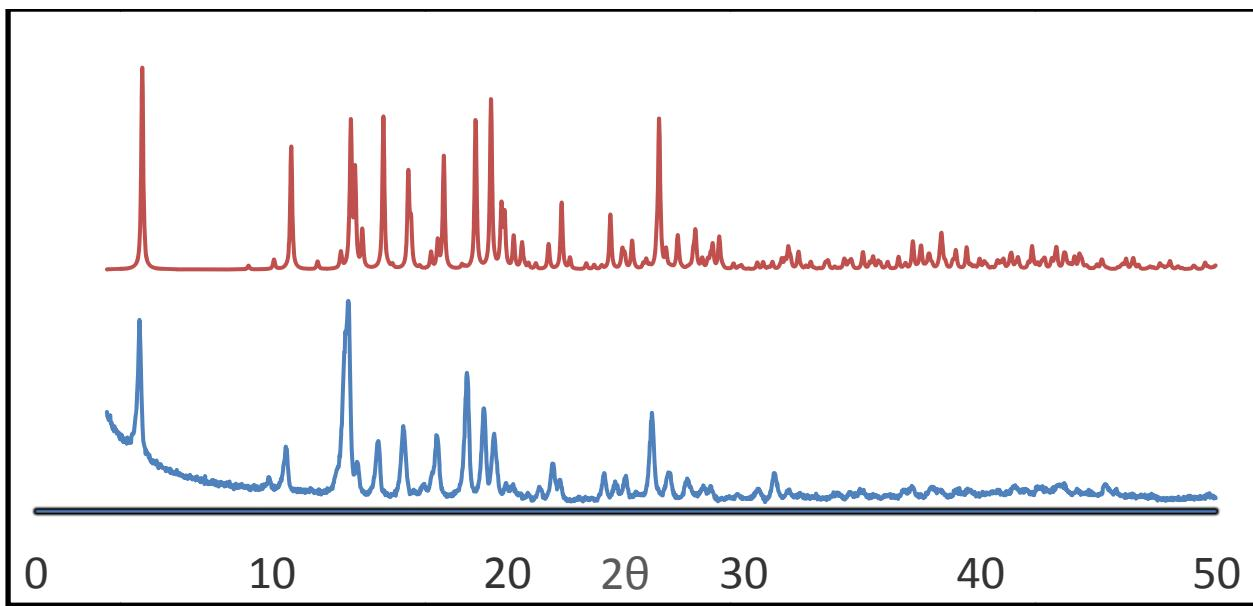
Figure S35: Powder XRD data of compound **4**. Experimental result (bottom, blue), simulated result from crystal structure (top, red).
