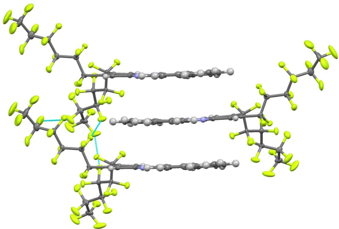
Figure S31: F-F short contact ( $C_{sp^3}$ -F-F- $C_{sp^3}$  attractive intermolecular interactions) observed between alternative molecules of **5** in crystal packing: (color code: light green, F; light blue, N; gray, C; white, H).
