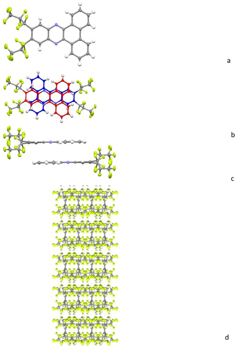
Figure S24: (a) Crystal structure, (b) topview dimer (overlapped dibenzphenazine rings are highlighted in red and blue colors, (c) sideview dimer, (d) crystal packing along b axis of **3**: (color code: light green, F; light blue, N; gray, C; white, H).
