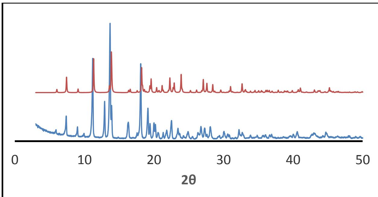
Figure S37: Powder XRD data of compound **7**. Experimental result (bottom, blue), simulated result from crystal structure (top, red).
