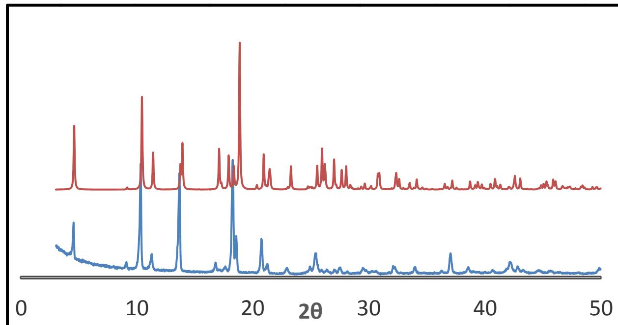
Figure S34: Powder XRD data of compound 3. Experimental result (bottom, blue), simulated result from crystal structure (top, red).
