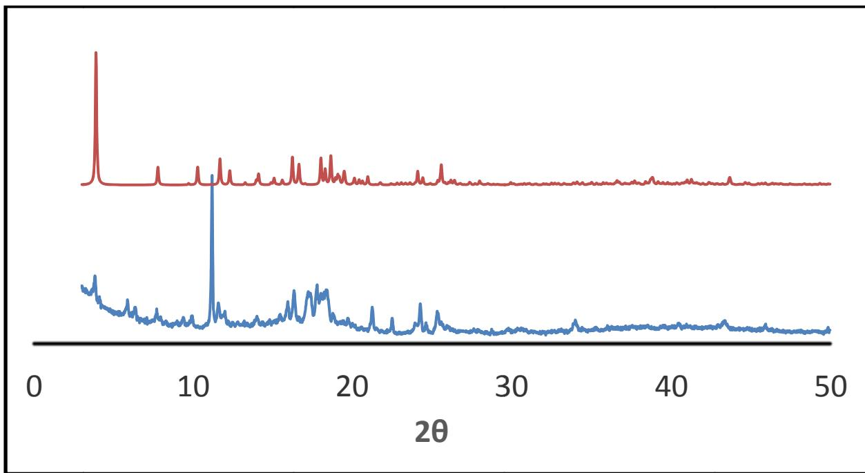
Figure S36: Powder XRD data of compound **5**. Experimental result (bottom, blue), simulated result from crystal structure (top, red).
