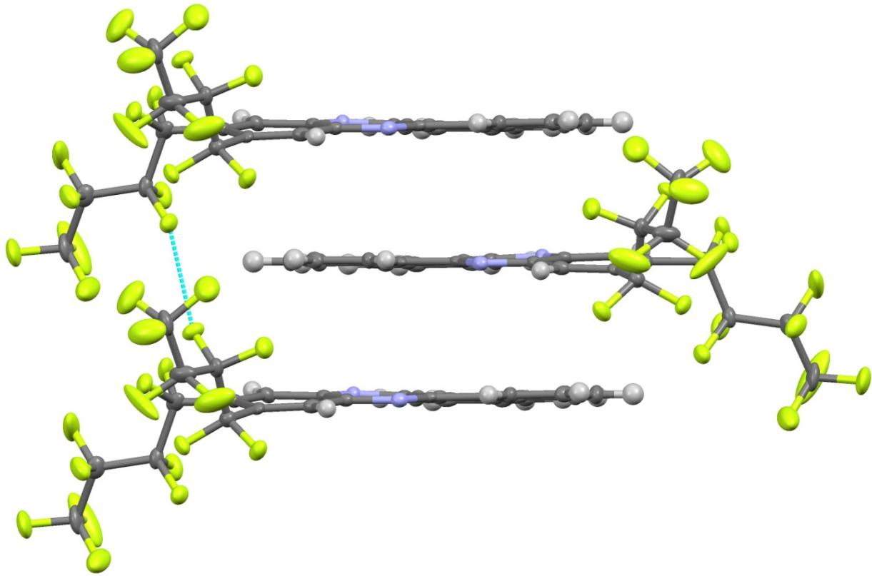
Figure S30: F-F short contact ( $C_{sp^3}$ -F-F- $C_{sp^3}$  attractive intermolecular interactions) observed between alternative molecules of **4** in crystal packing: (color code: light green, F; light blue, N; gray, C; white, H).
