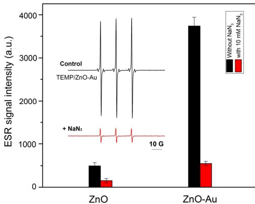
Figure S4. Effect of NaN<sub>3</sub> on ESR signal intensity from spin labels 4-Oxo-TEMP in the presence of ZnO or ZnO/Au hybrid nanostructures. (Conditions: 10 mM 4-Oxo-TEMP, 10 mM NaN<sub>3</sub>, 0.1 mg/ml ZnO or ZnO/Au hybrid nanostructures with Au/ZnO loading ratio 4%, irradiation for 3 min with simulated sunlight.)
