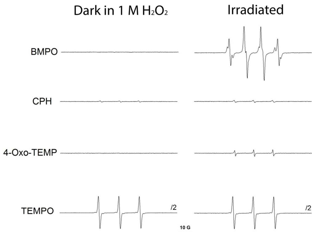
Figure S6. Effect of hydroxyl radicals on different spin probes. ESR spectra were obtained from samples containing 1 M H<sub>2</sub>O<sub>2</sub>, and different spin probes (25 mM BMPO, 10 mM 4-oxo-TEMP, 0.02 mM CPH and 0.02 mM TEMPO) in the dark or irradiated with simulated sunlight. Spectra were recorded at before and after irradiation for 3 min. The hydroxyl radical was generated by decomposition of hydrogen peroxide during exposure to UV radiation in simulated sunlight.
