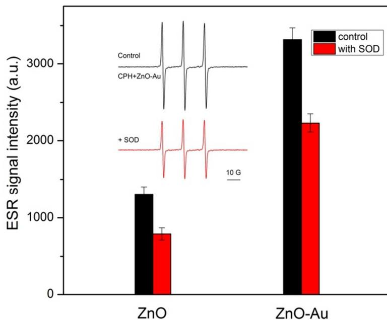
Figure S8. Effect of SOD on ESR signal intensity generated from CPH oxidation in the presence of ZnO or ZnO/Au hybrid nanostructures. (Conditions: 0.02 mM CPH, 0.25 U/ml SOD, 0.1 mg/ml ZnO or ZnO/Au hybrid nanostructures with a molar loading ratio of Au to ZnO of 4%, irradiation for 3 min with simulated sunlight.)
