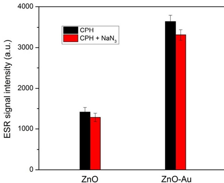
Figure S7. Effect of NaN<sub>3</sub> on ESR signal intensity from CPH in the presence of ZnO or ZnO/Au hybrid nanostructures. (Conditions: 0.02 mM CPH, 10 mM NaN<sub>3</sub>, 0.1 mg/ml ZnO or ZnO/Au hybrid nanostructures with Au/ZnO loading ratio 4%, irradiation for 3 min with simulated sunlight.)
