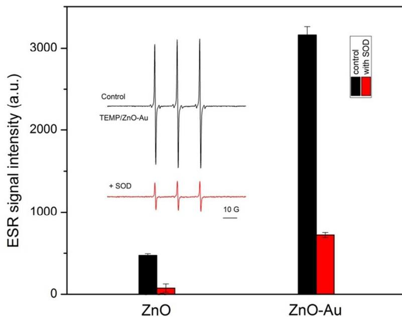
Figure S9. Effect of SOD on ESR signal intensity generated from spin labels 4-Oxo-TEMP in the presence of ZnO or ZnO/Au hybrid nanostructures. (Conditions: 10 mM 4-Oxo-TEMP, 0.25 U/ml SOD, 0.1 mg/ml ZnO or ZnO/Au hybrid nanostructures with a molar loading ratio of Au to ZnO of 4%, irradiation for 3 min with simulated sunlight.)
