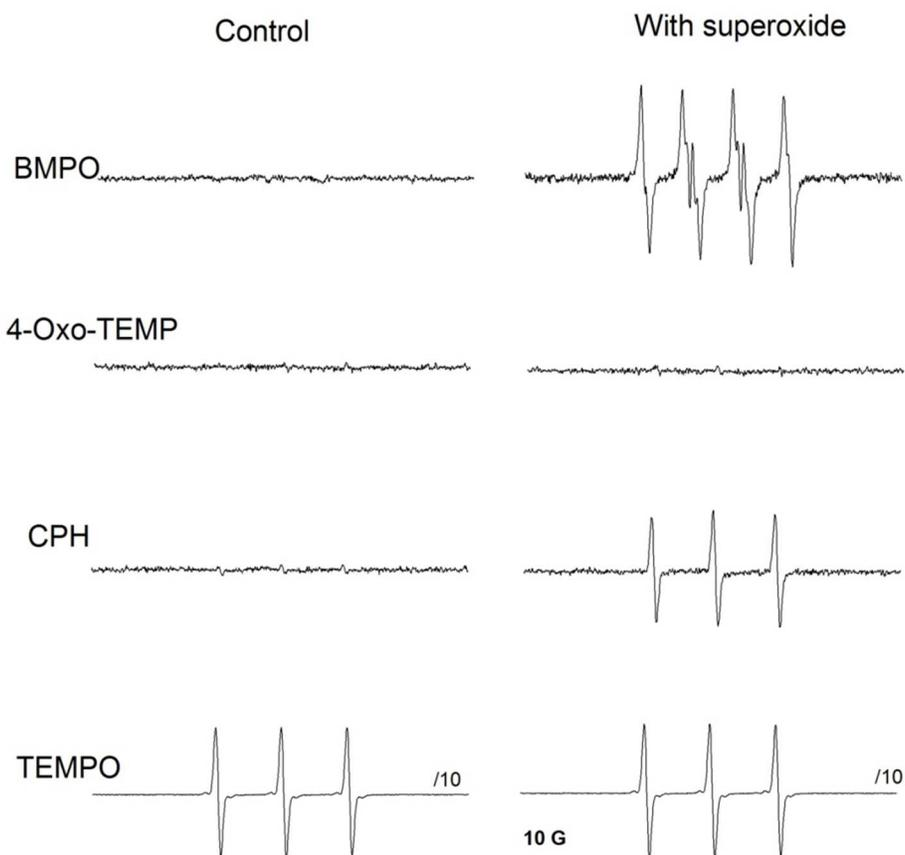
Figure S5. Effect of superoxide on different spin probes. The conditions used to form superoxide are same as in Figure S3. The control spectra were obtained from samples containing 0.05 mM DTPA, 1 mM xanthine and 25 mM BMPO (or 10 mM 4-Oxo-TEMP, or 0.02 mM CPH, or 0.02 mM TEMPO) before adding 0.2U/ml XOD to initiate the generation of superoxide.
