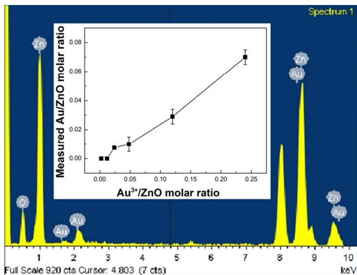
Figure S1. Energy-dispersive X-ray (EDX) analysis of ZnO/Au hybrid nanoparticles. Inset: Effect of the added  $\text{HAuCl}_4^-/\text{ZnO}$  molar ratio on the obtained Au/ZnO molar ratio in the nanostructures measured by EDX analysis. Au/ZnO ratio from EDX vs  $\text{HAuCl}_4^-/\text{ZnO}$  ratio.
