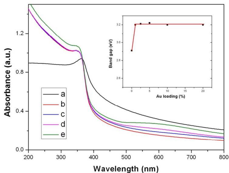
Figure S2. UV-Vis spectra of ZnO (a) and various ZnO/Au hybrid nanostructures formed at different  $\text{HAuCl}_4^-/\text{ZnO}$  molar ratios of 0.2% (b), 1.0% (c), 2.0 (d) and 4.0% (e). Inset: band gap
