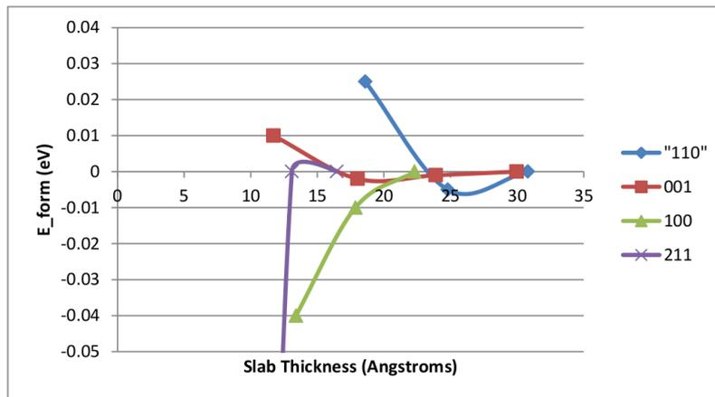
Figure S4: Calculated defect formation energies as a function of slab thickness. The zero reference formation energy is set to that calculated for the greatest slab thickness used for each surface.
