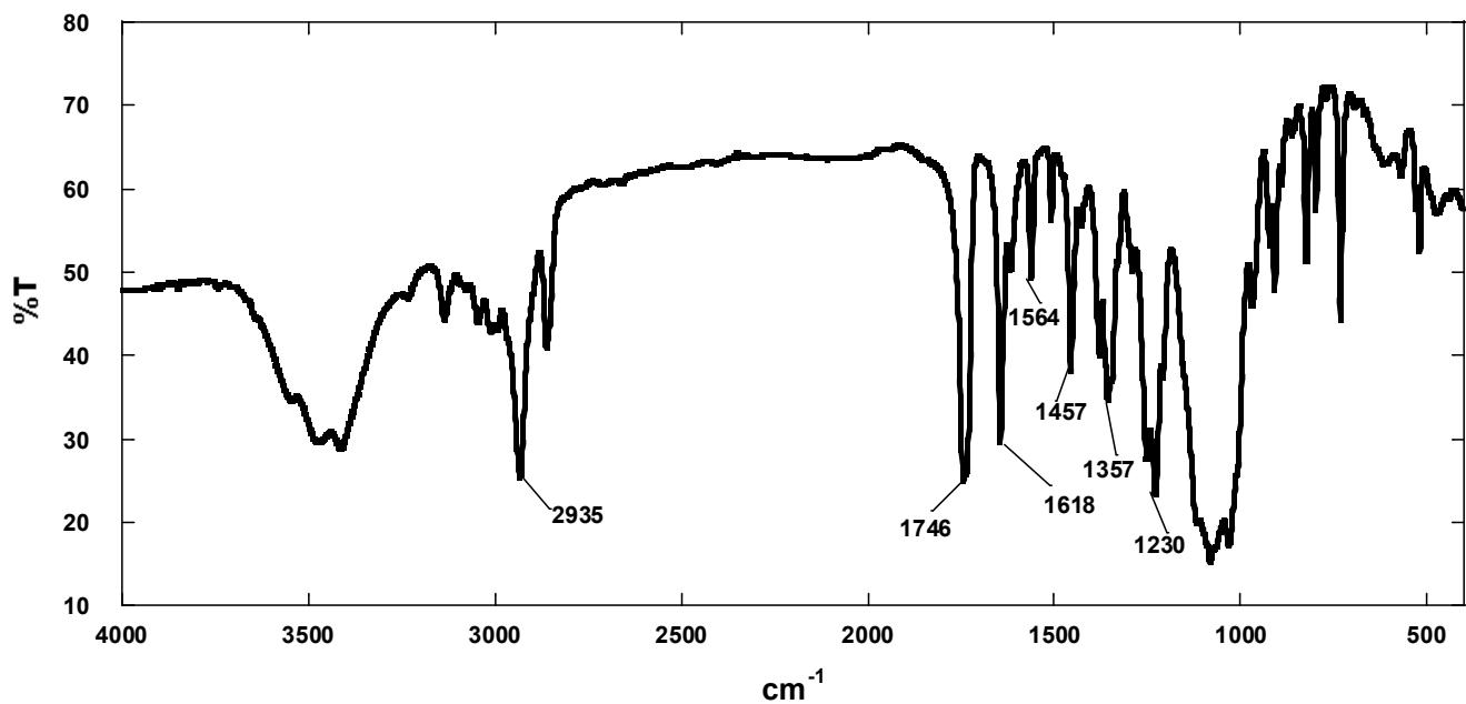
IR spectra of 1,1'-bis-(2-(cyclohexyloxy)-2-oxoethyl)-[4,4'-bipyridin]-1,1'-diium tetrafluoroborate (11b)
