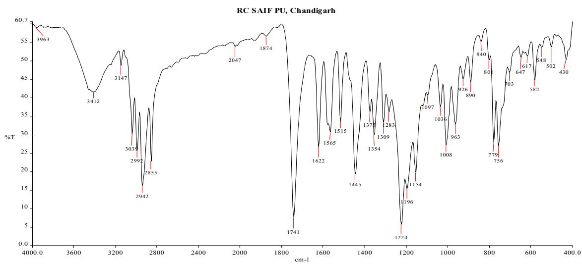
**IR spectra of 1,1'-bis-(2-(cyclohexyloxy)-2-oxoethyl)-[2,2'-bipyridin]-1,1'-diium bromide (7b)**
