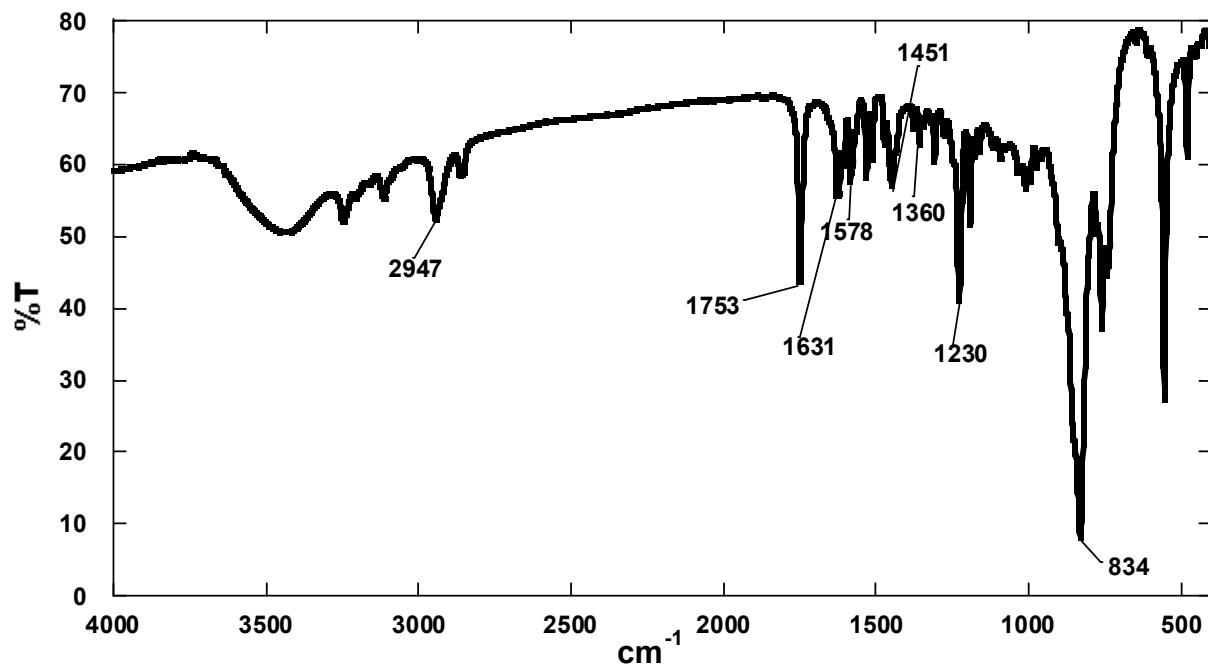
IR spectra of 1,1'-bis-(2-(cyclohexyloxy)-2-oxoethyl)-[2,2'-bipyridin]-1,1'-diium hexafluorophosphate (12a)
