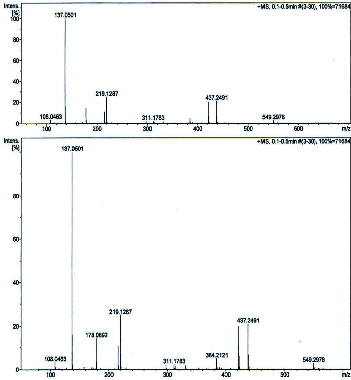
Mass spectra of 1,1'-bis-(2-(cyclohexyloxy)-2-oxoethyl)-[4,4'-bipyridin]-1,1'-diium chloride (6a)
