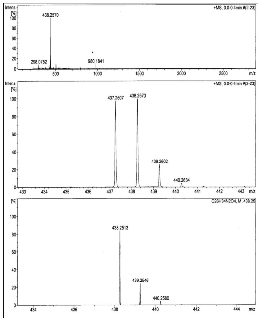
**Mass spectra of 1,1'-bis-(2-(cyclohexyloxy)-2-oxoethyl)-[2,2'-bipyridin]-1,1'-diium chloride (7a)**
