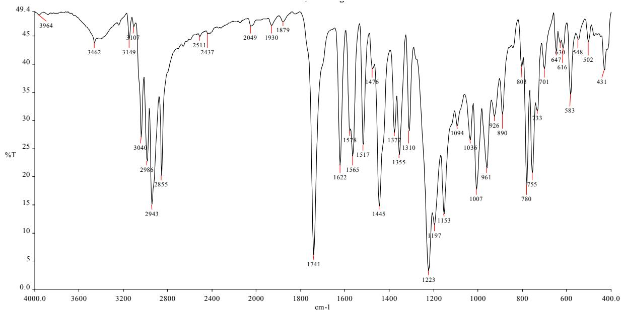
**IR spectra of 1,1'-bis-(2-(cyclohexyloxy)-2-oxoethyl)-[2,2'-bipyridin]-1,1'-diium chloride (7a)**
