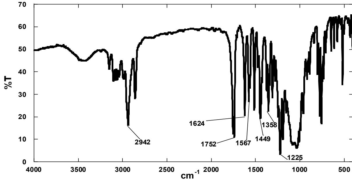
IR spectra of 1,1'-bis-(2-(cyclohexyloxy)-2-oxoethyl)-[2,2'-bipyridin]-1,1'-diium tetrafluoroborate (12b)
