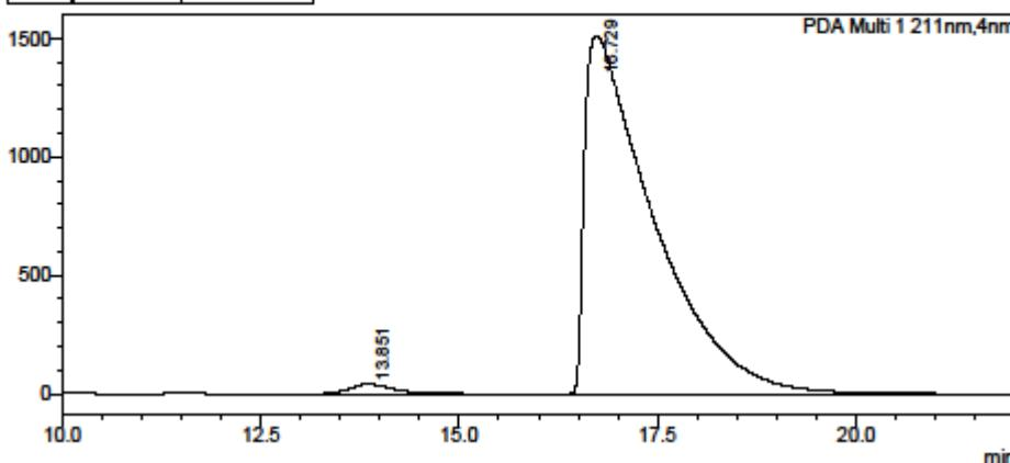
HPLC data compound **42**: Chiral HPLC Chiraldak IB (5% IPA:hexane, flow rate 1 mL min<sup>-1</sup>, 211 nm, 30 °C) t<sub>R</sub>(2S): 11.3 min, t<sub>R</sub>(2R): 15.6 min, 99% ee.
