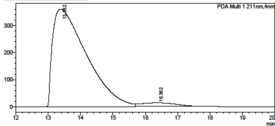
HPLC data compound **41**: Chiral HPLC Chiraldak IB (5% IPA:hexane, flow rate 1 mL min<sup>-1</sup>, 211 nm, 30 °C) t<sub>R</sub>(2S): 13.2 min, t<sub>R</sub>(2R): 17.3 min, 96% ee.
