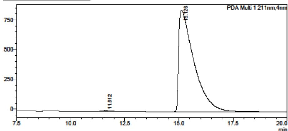
HPLC data compound **43**: Chiral HPLC Chiraldpak IB (5% IPA:hexane, flow rate 1 mL min<sup>-1</sup>, 211 nm, 30 °C) t<sub>R</sub>(2S): 14.5 min, t<sub>R</sub>(2R): 19.0 min, 99% ee.
