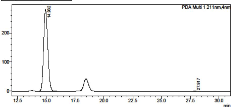
HPLC data compound **77**: Chiral HPLC Chiraldpak AD-H (10% IPA:hexane, flow rate 1 mL min<sup>-1</sup>, 211 nm, 30 °C) t<sub>R</sub>(3*S*,4*S*): 14.4 min, t<sub>R</sub>(3*R*,4*R*): 26.7 min, 39% *ee* at rt and 97% *ee* at -78 °C.
