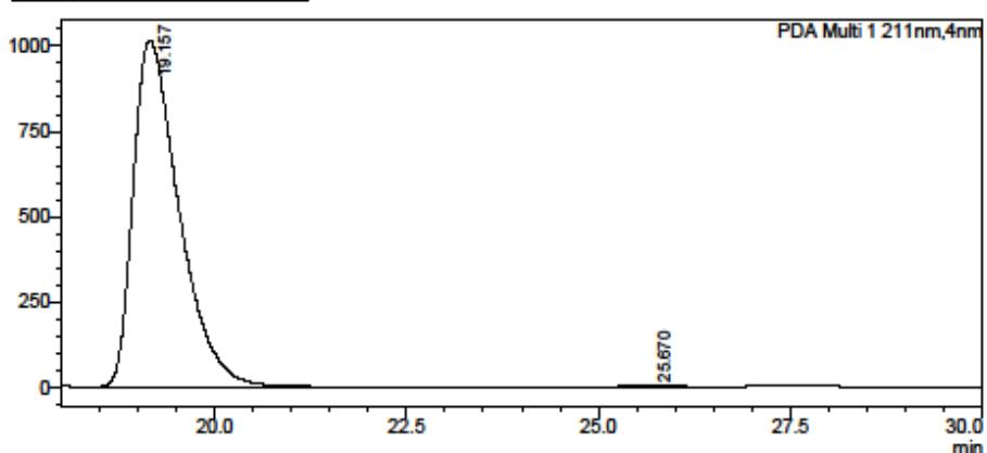
HPLC data compound **76**: Chiral HPLC Chiraldpak AD-H (10% IPA:hexane, flow rate 1 mL min<sup>-1</sup>, 211 nm, 30 °C) t<sub>R</sub>(3S,4S): 14.9 min, t<sub>R</sub>(3R,4R): 27.9 min, 74% ee at rt and >99% ee at -78 °C.
