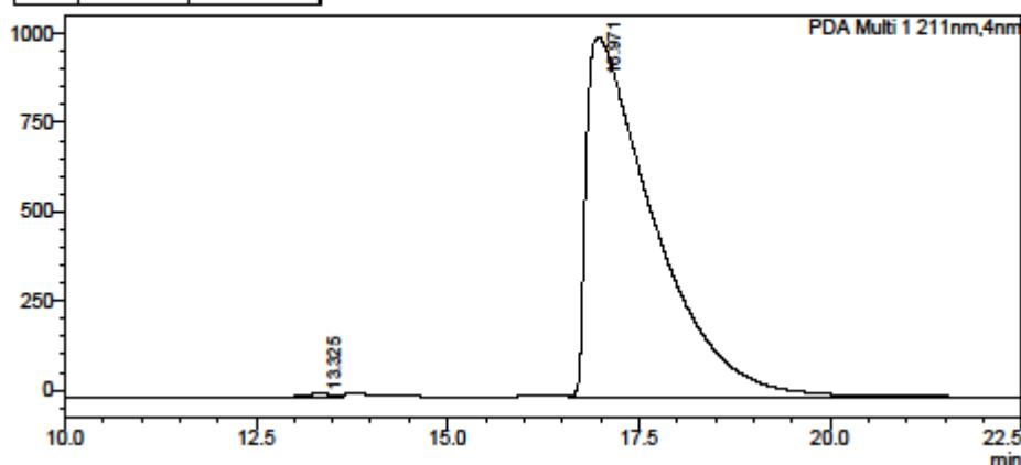
HPLC data compound **48**: Chiral HPLC Chiraldak IB (5% IPA:hexane, flow rate 1 mL min<sup>-1</sup>, 211 nm, 30 °C) t<sub>R</sub>(2S): 16.0 min, t<sub>R</sub>(2R): 22.2 min, 99% ee.
