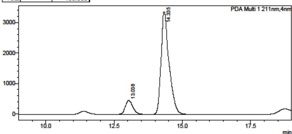
HPLC data compound **74**: Chiral HPLC Chiraldpak AD-H (10% IPA:hexane, flow rate 1 mL min<sup>-1</sup>, 211 nm, 30 °C) t<sub>R</sub>(3*S*,4*S*): 23.0 min, t<sub>R</sub>(3*R*,4*R*): 46.8 min, 16% ee at -78 °C.
