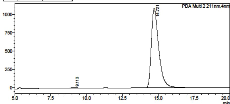
HPLC data compound **73**: Chiral HPLC Chiralcel OD-H (2% IPA:hexane, flow rate 1 mL min<sup>-1</sup>, 211 nm, 30 °C) t<sub>R</sub>(3*S*,4*S*): 13.1 min, t<sub>R</sub>(3*R*,4*R*): 14.9 min, 77% *ee* at rt.
