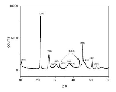
Figure S2. XRD spectrum of crystal synthesized by non-stoichiometric melt
