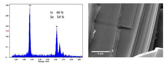
**Figure S1.** EDX spectra (left) and SEM image (right) of InSe crystal synthesized by nonstoichiometric melt method. EDX shows an elemental ratio of 1 :1 between In and Se. SEM image shows an obvious layered structure.
