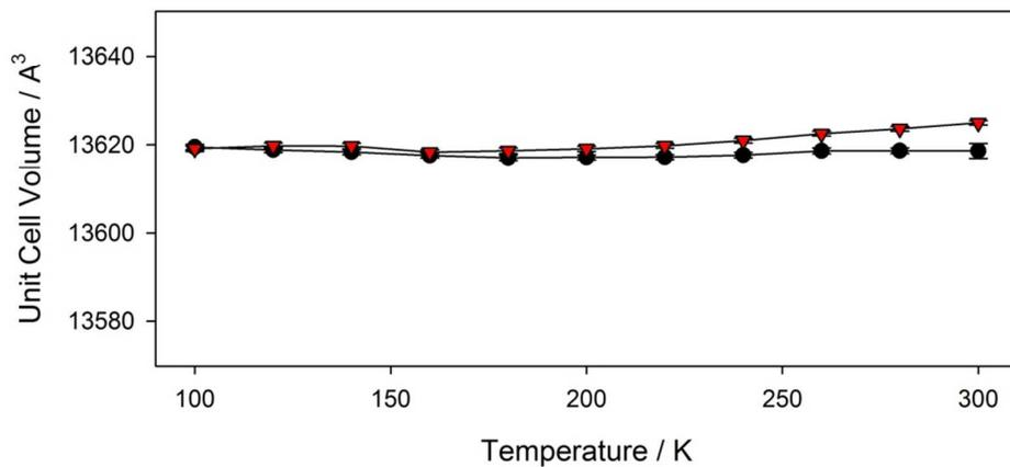
Figure 5 – Calculated unit cell volumes of dehydrated Li-A from 100–300 K.
