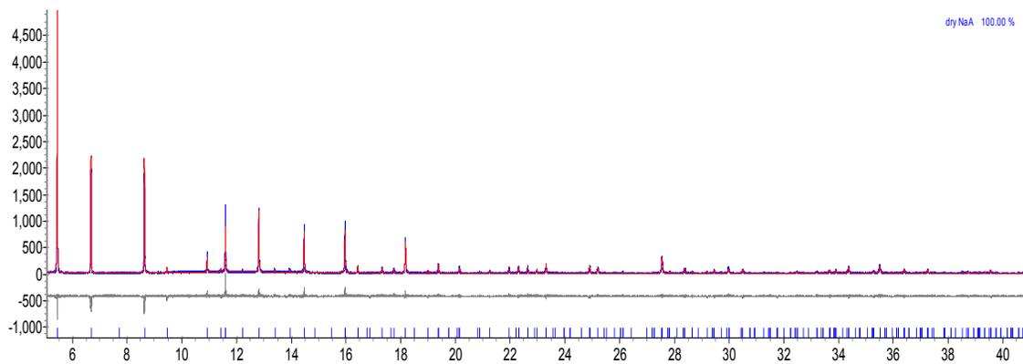
Figure 25 - Rietveld refinement plot of dehydrated Na-A at 200 K.
