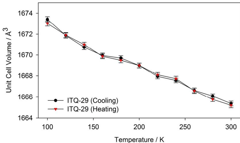
Figure 1 – Calculated unit cell volumes of ITQ-29 from 100–300 K.
