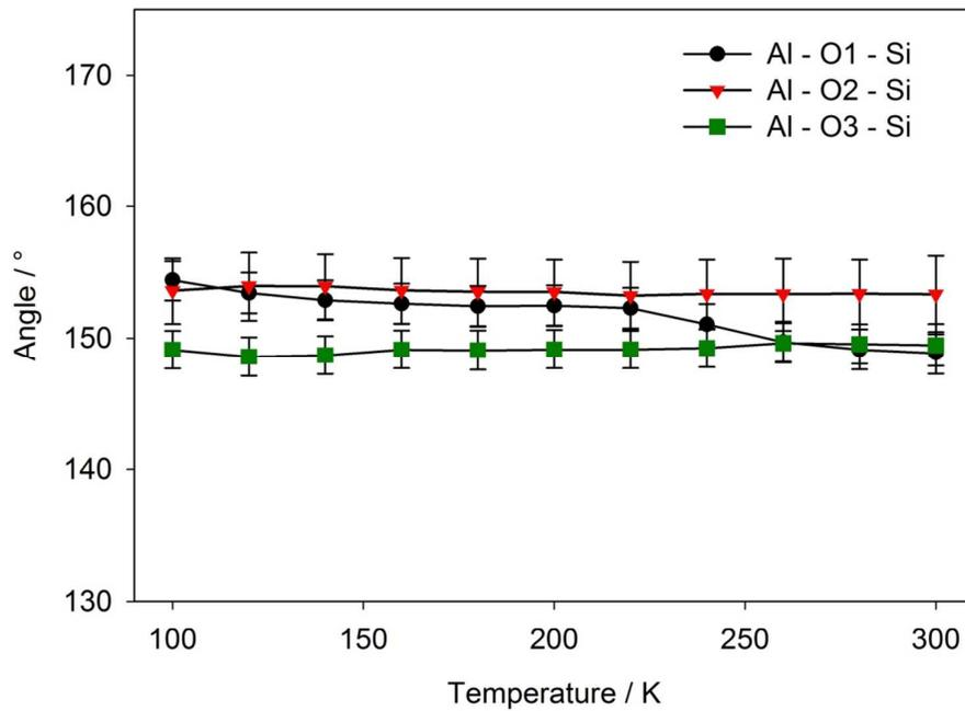
Figure 4 – Calculated Si–O–Al bond angles for dehydrated Ag-A from 100–300 K.
