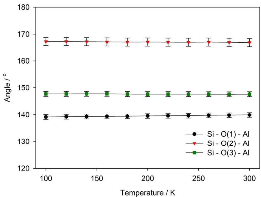
Figure 10 – Calculated Si–O–Al bond angles for dehydrated  $\text{Rb}_{0.79}\text{Na}_{0.21}\text{-A}$  from 100–300 K.
