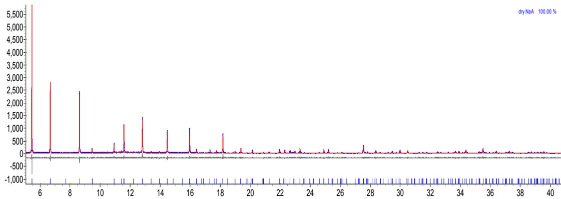
Figure 24 - Rietveld refinement plot of dehydrated Na-A at 300 K.
