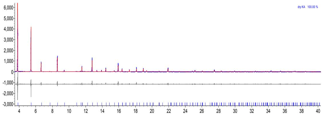
Figure 28 - Rietveld refinement plot of dehydrated K-A at 200 K.
