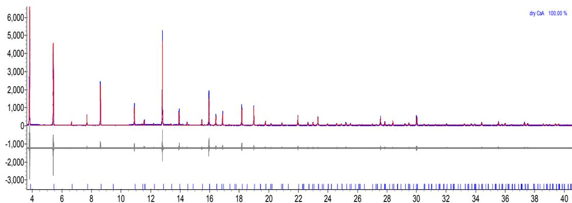
Figure 35 - Rietveld refinement plot of dehydrated Cs<sub>0.58</sub>Na<sub>0.42</sub>-A at 100 K.
