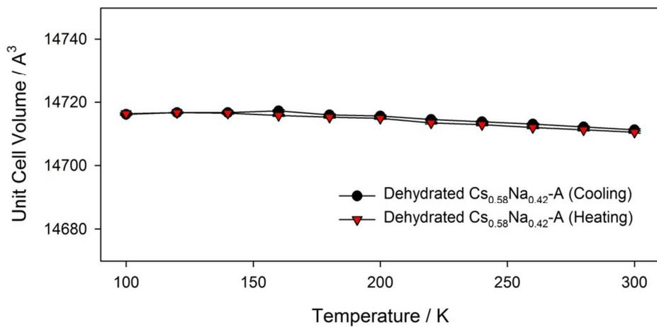
Figure 12 – Calculated unit cell volumes of dehydrated  $\text{Cs}_{0.58}\text{Na}_{0.42}\text{-A}$  from 100–300 K.
