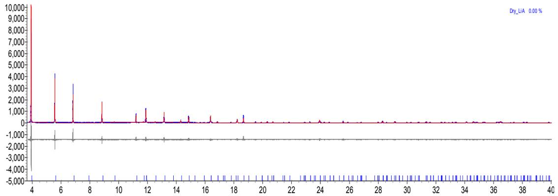
Figure 21 - Rietveld refinement plot of dehydrated Li-A at 300 K.
