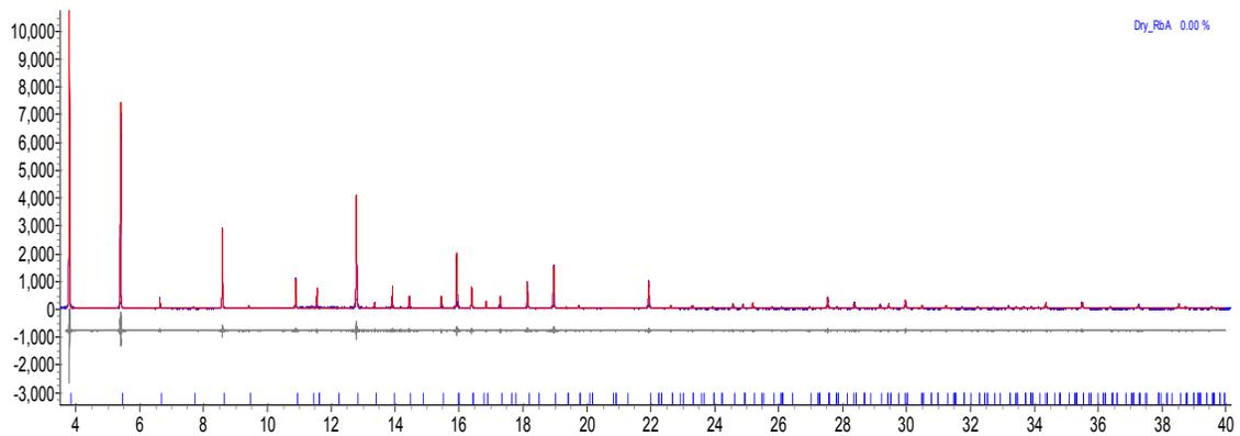
Figure 31 - Rietveld refinement plot of dehydrated  $\text{Rb}_{0.79}\text{Na}_{0.21}\text{-A}$  at 200 K.
