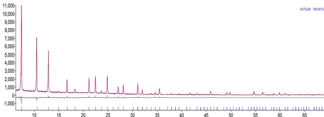
Figure 15 - Rietveld refinement plot of ITQ-29 at 300 K.
