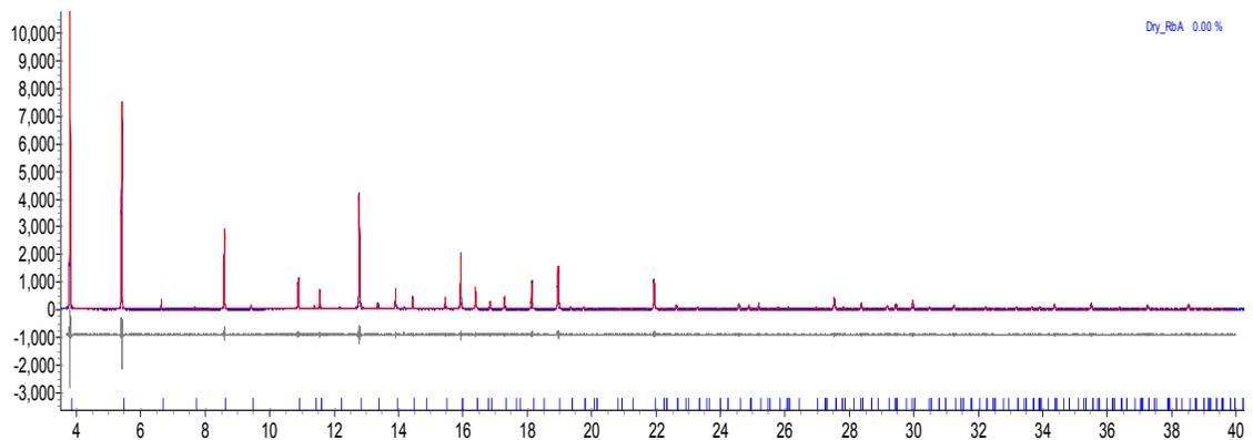
Figure 32 - Rietveld refinement plot of dehydrated  $\text{Rb}_{0.79}\text{Na}_{0.21}\text{-A}$  at 100 K.
