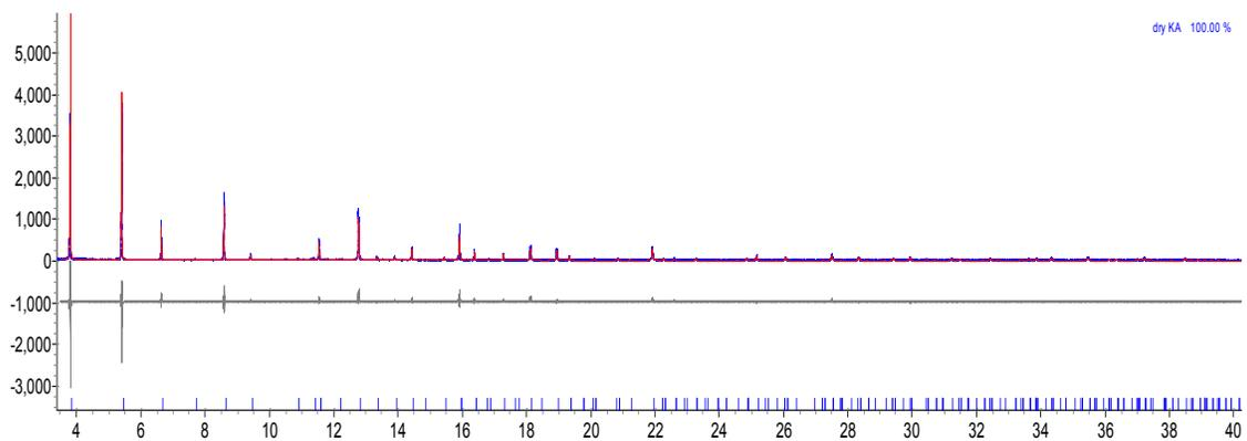
Figure 29 - Rietveld refinement plot of dehydrated K-A at 100 K.
