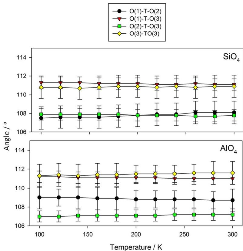
Figure 11 - Calculated O-T-O bond angles for dehydrated  $\text{Rb}_{0.79}\text{Na}_{0.21}\text{-A}$  from 100–300 K.
