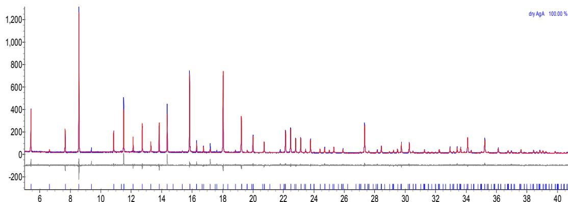
Figure 20 - Rietveld refinement plot of dehydrated Ag-A at 100 K.
