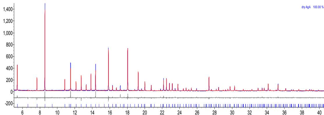
Figure 18 - Rietveld refinement plot of dehydrated Ag-A at 300 K.
