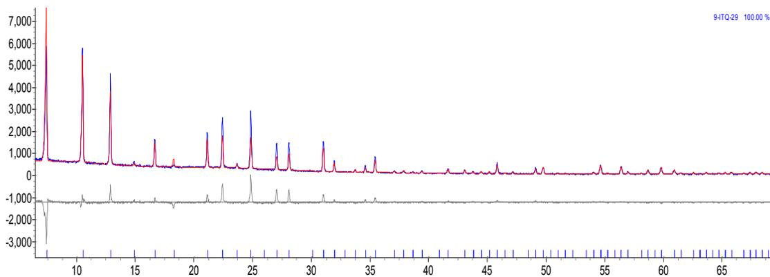
Figure 17 - Rietveld refinement plot of ITQ-29 at 100 K.
