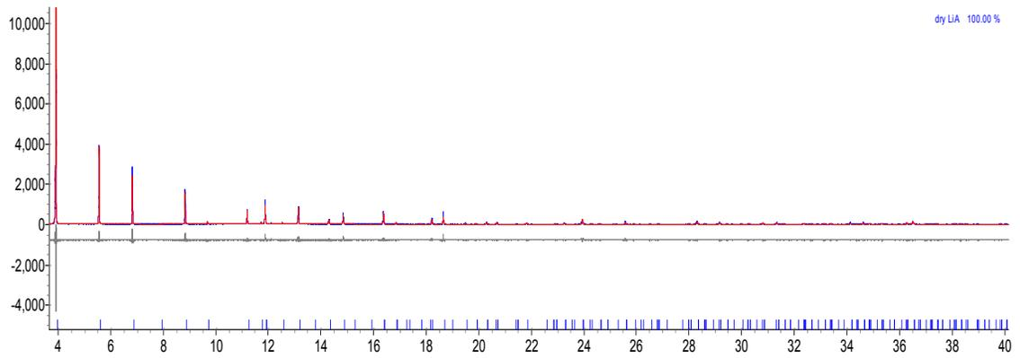
Figure 22 - Rietveld refinement plot of dehydrated Li-A at 200 K.
