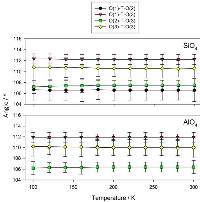
Figure 14 - Calculated O-T-O bond angles for dehydrated  $\text{Cs}_{0.58}\text{Na}_{0.42}\text{-A}$  from 100–300 K.
