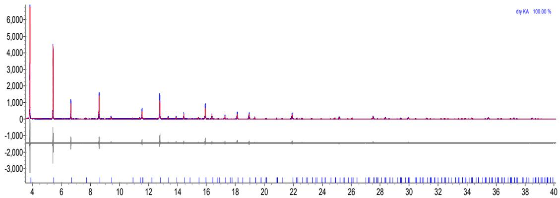
Figure 27 - Rietveld refinement plot of dehydrated K-A at 300 K.
