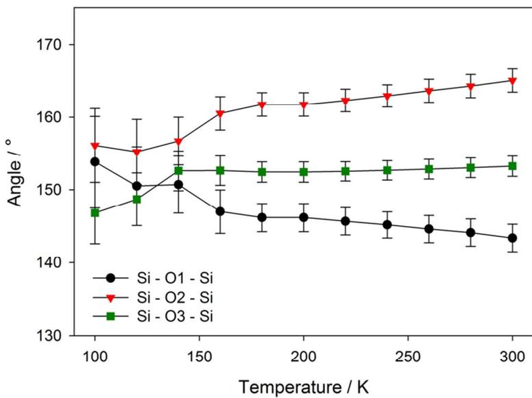
Figure 2 – Calculated Si-O-Si bond angles for ITQ-29 from 100–300 K.
