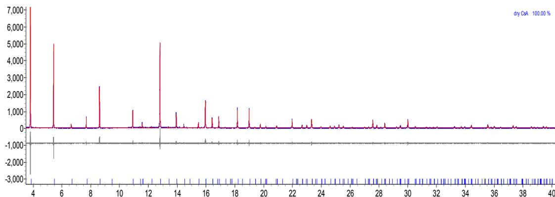
Figure 34 - Rietveld refinement plot of dehydrated Cs<sub>0.58</sub>Na<sub>0.42</sub>-A at 200 K.
