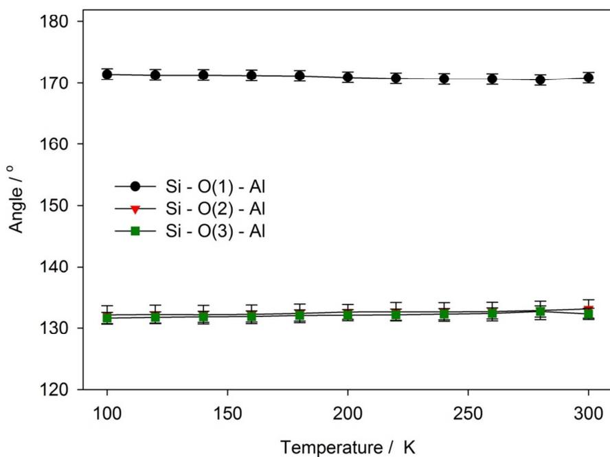
Figure 6 – Calculated Si–O–Al bond angles for dehydrated Li-A from 100–300 K.
