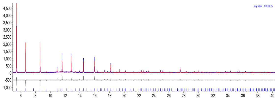
Figure 26 - Rietveld refinement plot of dehydrated Na-A at 100 K.
