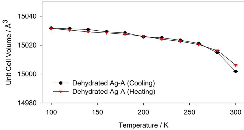
Figure 3 – Calculated unit cell volumes of dehydrated Ag-A from 100–300 K.
