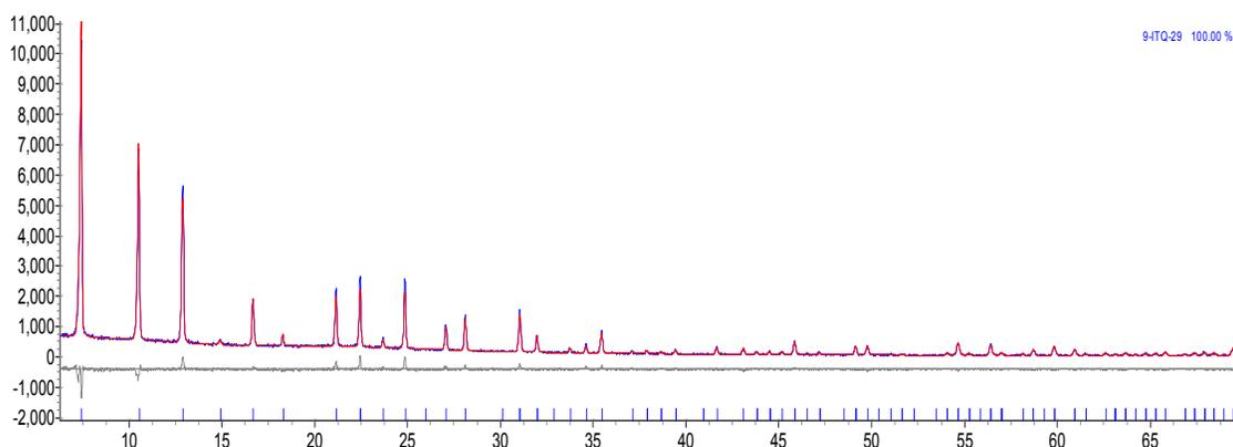
Figure 16 - Rietveld refinement plot of ITQ-29 at 200 K.
