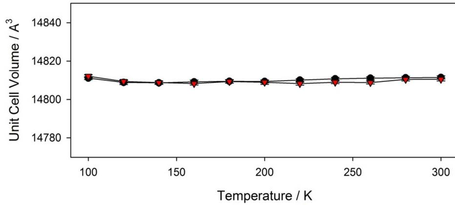
Figure 7 – Calculated unit cell volumes of dehydrated K-A from 100–300 K.
