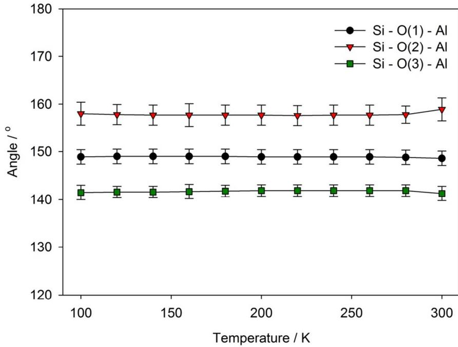
Figure 13 – Calculated Si–O–Al bond angles for dehydrated  $\text{Cs}_{0.58}\text{Na}_{0.42}\text{-A}$  from 100–300 K.
