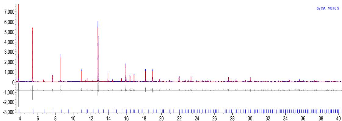
Figure 33 - Rietveld refinement plot of dehydrated Cs<sub>0.58</sub>Na<sub>0.42</sub>-A at 300 K.
