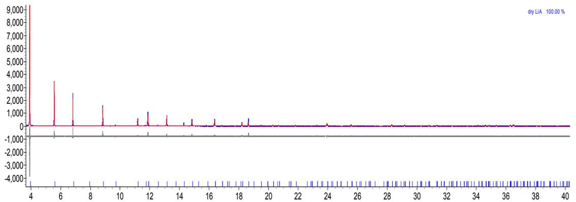
Figure 23 - Rietveld refinement plot of dehydrated Li-A at 100 K.
