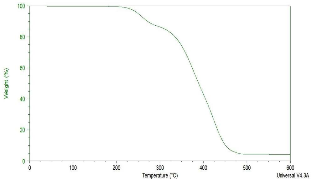
**Fig. S87** TGA curve of IM(1O2)24-TFSA.
