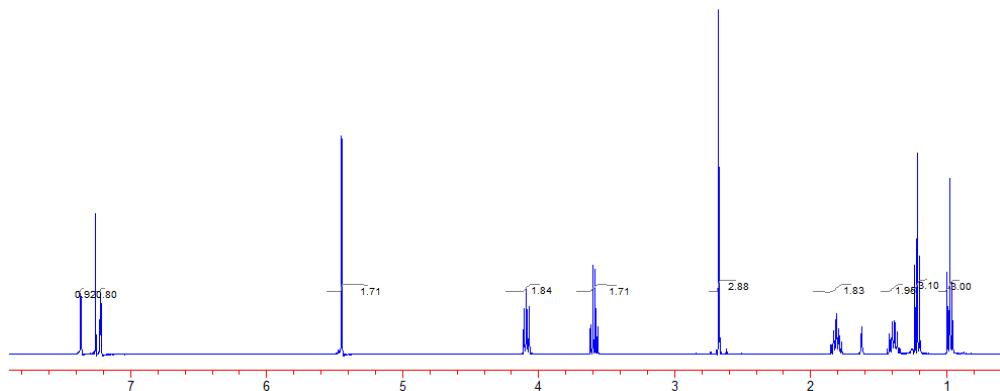
**Fig. S35**  $^1\text{H}$  NMR spectrum of IM(1O2)14-TFSA.
