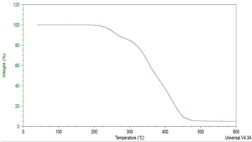
**Fig. S89** TGA curve of IM(1O2)2(2O2)-TFSA.
