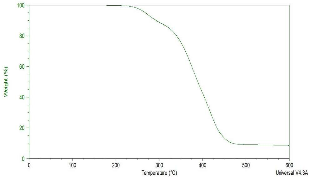
**Fig. S75** TGA curve of IM(1O1)24-TFSA.
