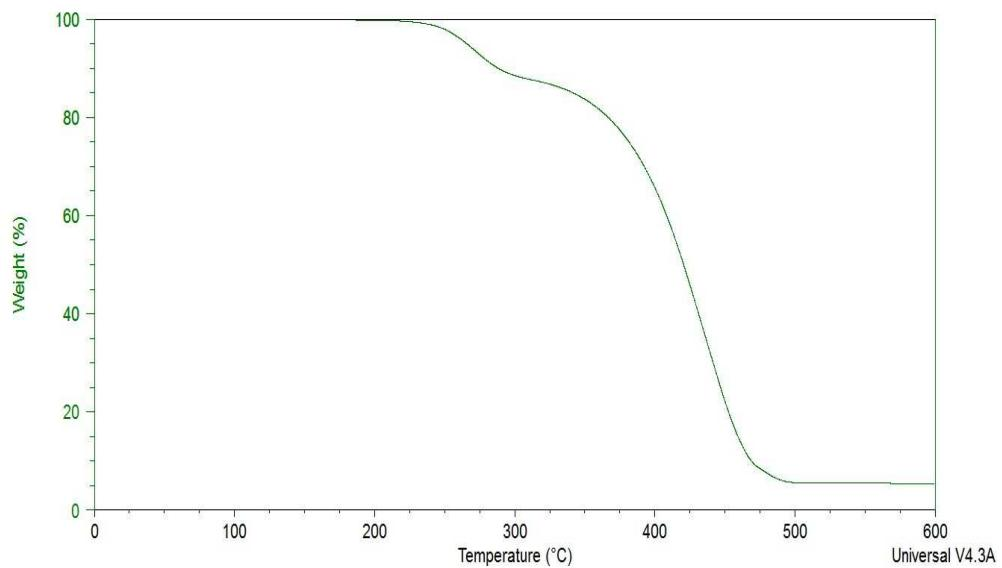
**Fig. S81** TGA curve of IM(1O2)14-TFSA.
