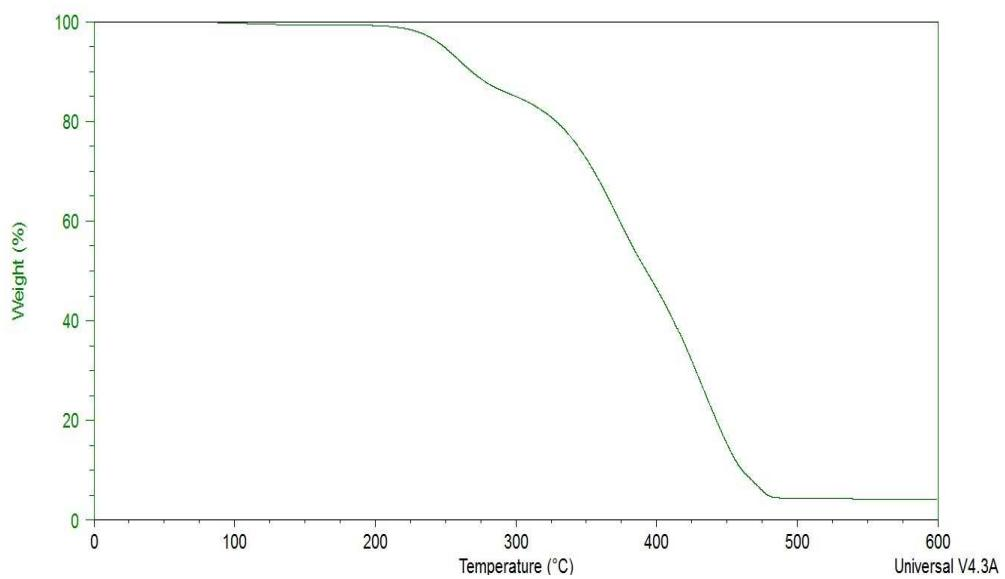
**Fig. S86** TGA curve of IM(1O2)23-TFSA.
