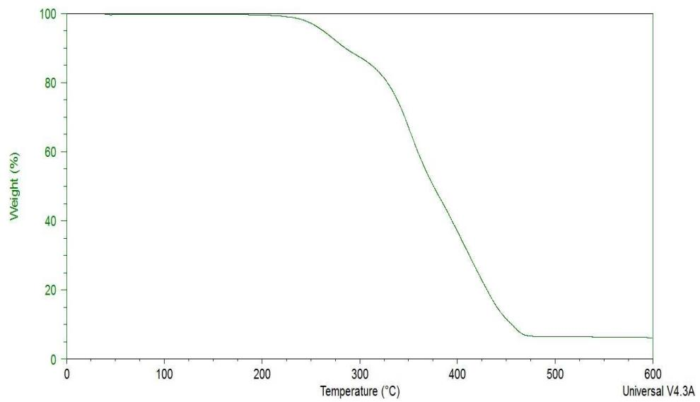
**Fig. S84** TGA curve of IM(1O2)21-TFSA.
