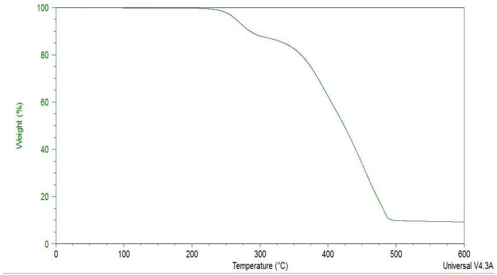
**Fig. S71** TGA curve of IM(1O1)1(2O2)-TFSA.
