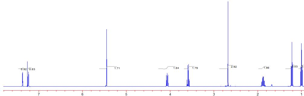
**Fig. S33** <sup>1</sup>H NMR spectrum of IM(1O2)13-TFSA.
