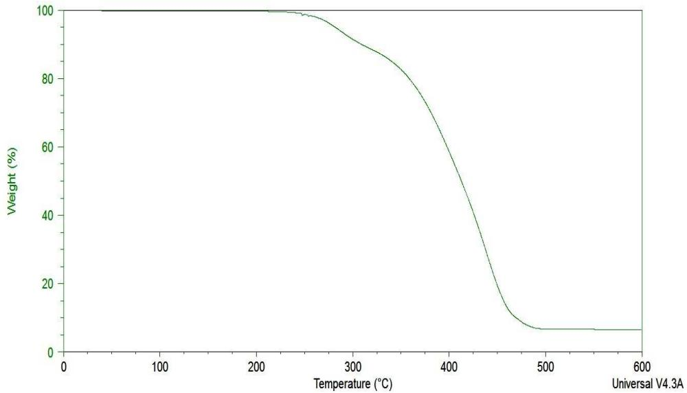
**Fig. S69** TGA curve of IM(1O1)14-TFSA.
