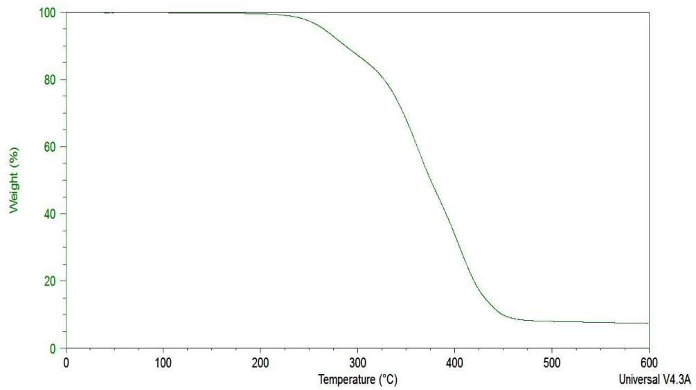
**Fig. S76** TGA curve of IM(1O1)2(2O1)-TFSA.
