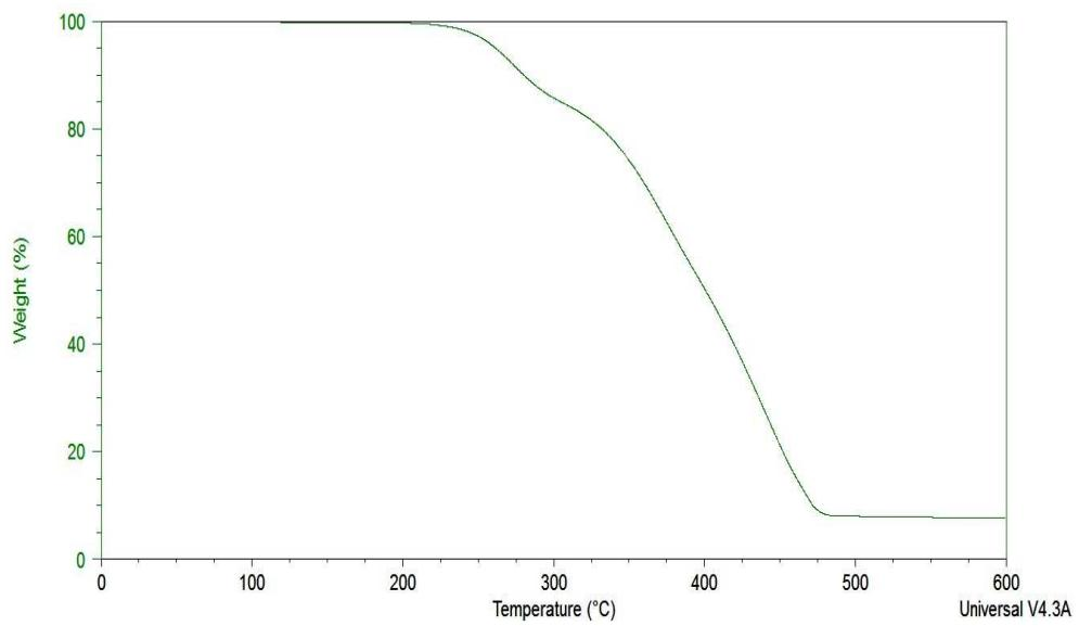
**Fig. S80** TGA curve of IM(1O2)13-TFSA.
