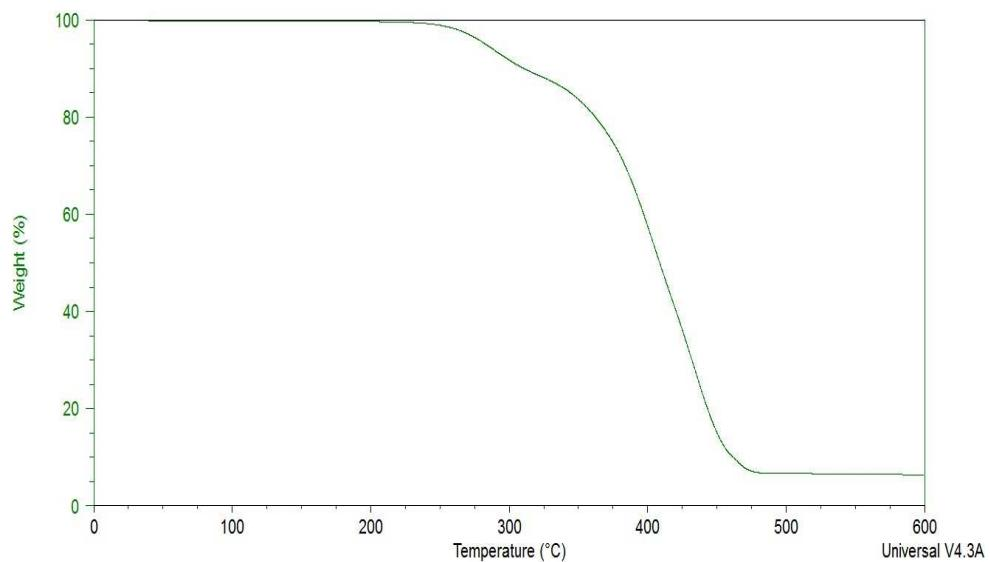
**Fig. S70** TGA curve of IM(1O1)1(2O1)-TFSA.
