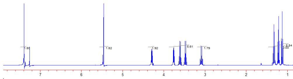
**Fig. S51**  $^1\text{H}$  NMR spectrum of IM(1O2)2(2o2)-TFSA.
