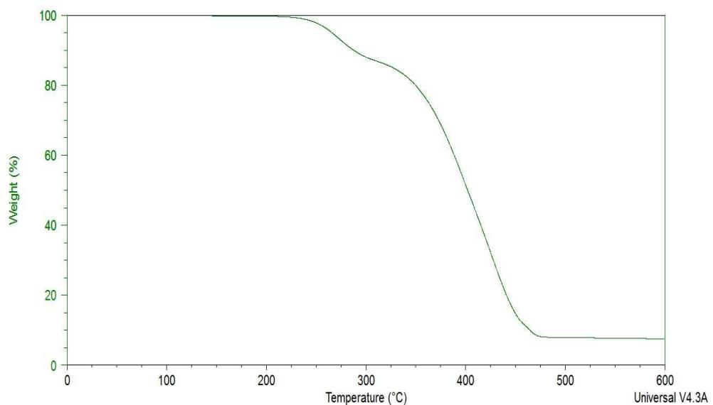
**Fig. S82** TGA curve of IM(1O2)1(2O1)-TFSA.
