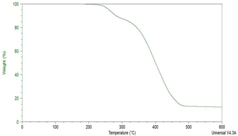
**Fig. S83** TGA curve of IM(1O2)1(2O2)-TFSA.
