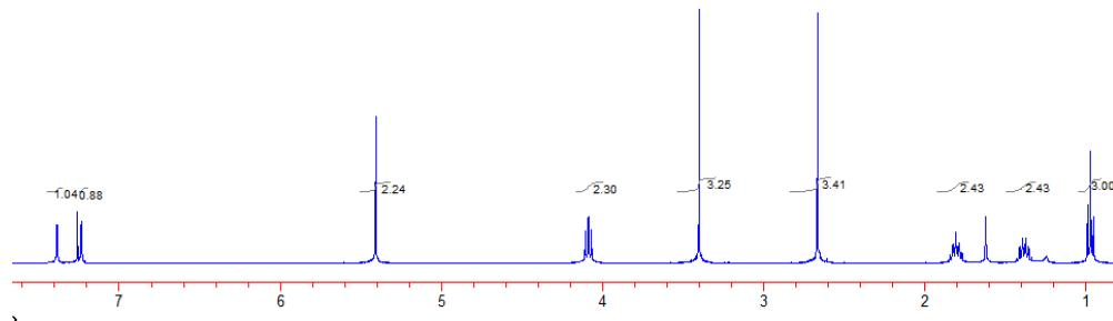
**Fig. S11**  $^1\text{H}$  NMR spectrum of IM(1O1)14-TFSA.
