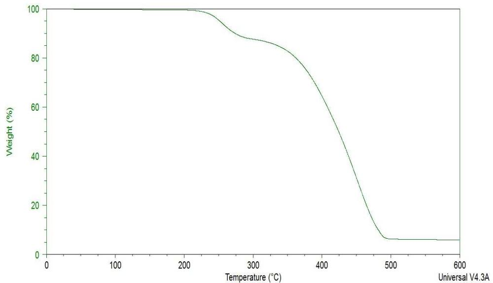
**Fig. S85** TGA curve of IM(1O2)22-TFSA.
