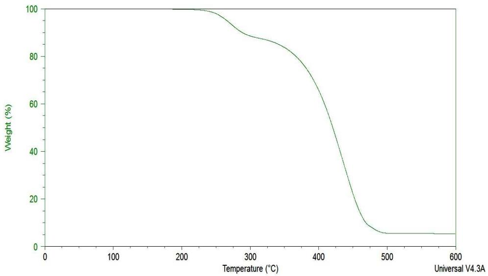
**Fig. S78** TGA curve of IM(1O2)11-TFSA.
