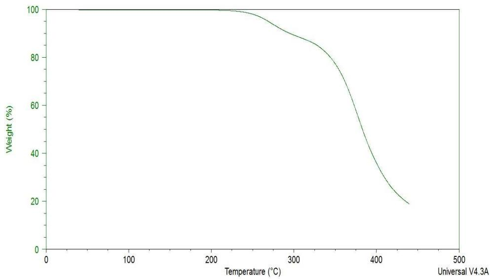
**Fig. S74** TGA curve of IM(1O1)23-TFSA.
