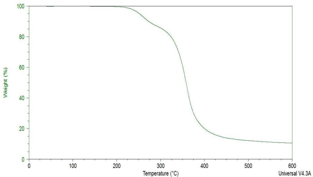
**Fig. S88** TGA curve of IM(1O2)2(2O1)-TFSA.
