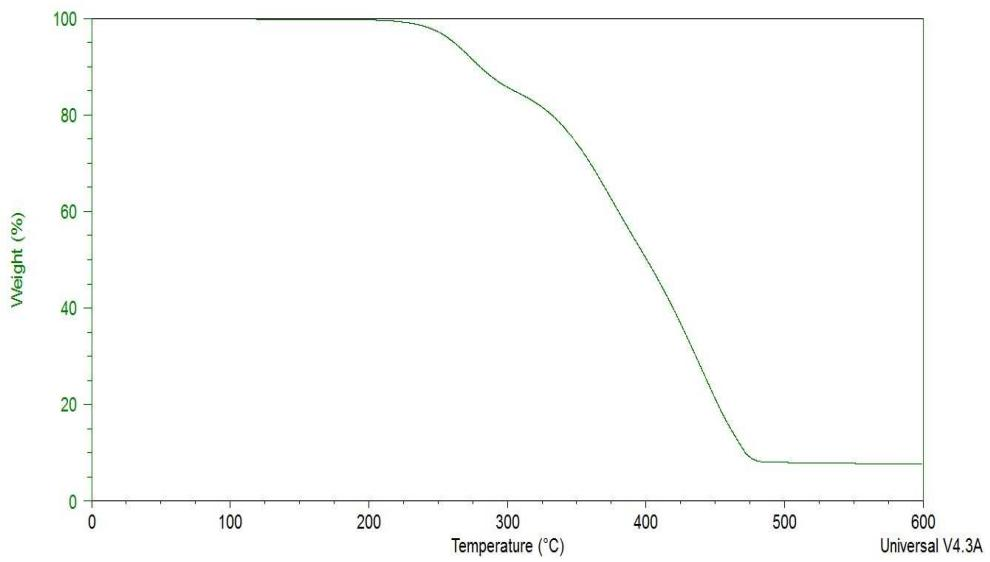
**Fig. S72** TGA curve of IM(1O1)21-TFSA.
