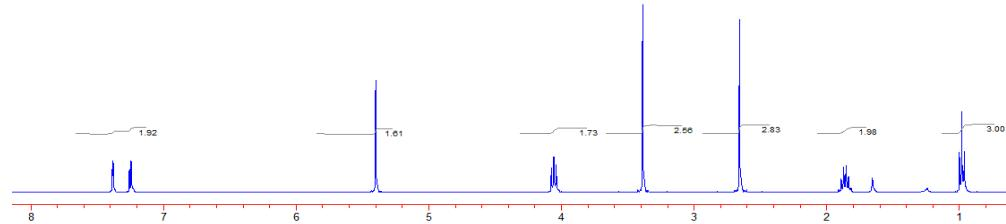
**Fig. S9** <sup>1</sup>H NMR spectrum of IM(1O1)13-TFSA.
