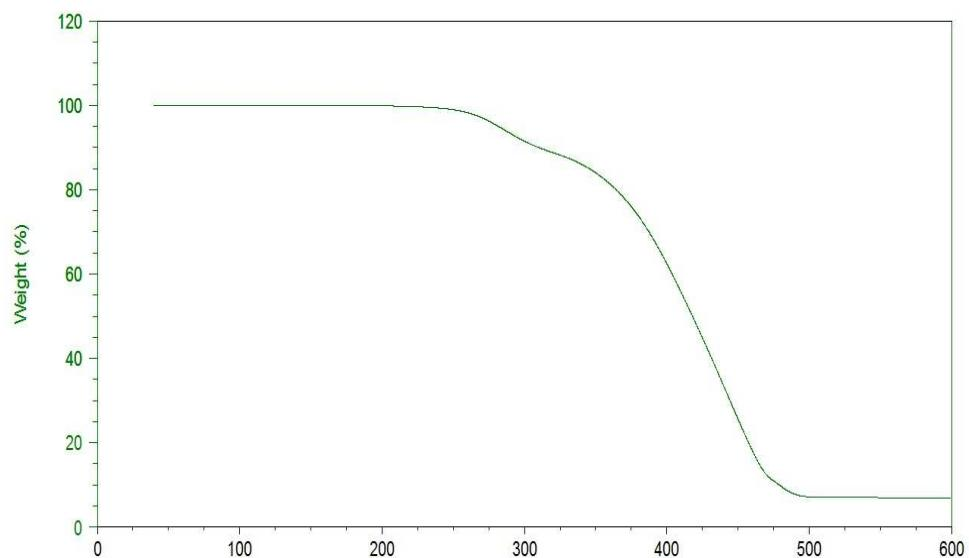
**Fig. S68** TGA curve of IM(1O1)13-TFSA.
