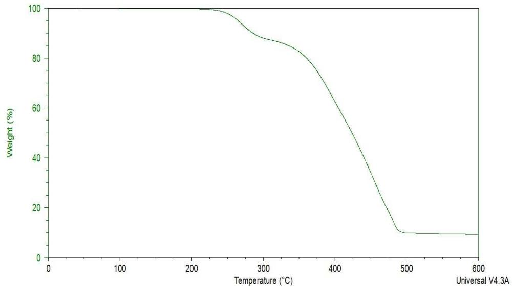
**Fig. S79** TGA curve of IM(1O2)12-TFSA.
