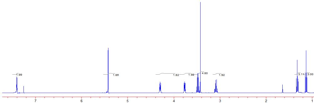
**Fig. S27**  $^1\text{H}$  NMR spectrum of IM(1O1)2(2o2)-TFSA.
