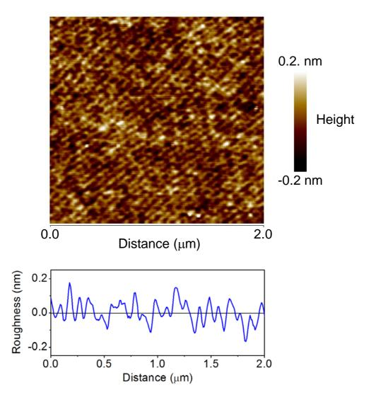
**Figure S1.** AFM image and surface profile of a representative a-Al<sub>2</sub>O<sub>3</sub> buffer layer produced by PLD in vacuum.
