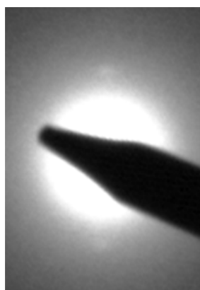
Figure S13. The central part of the diffraction pattern (here taken with a longer camera length) helps visualize the diffraction peaks due to the stacked lamellae. The periodicity of the lamellar thickness L is here 53 Å. Only the second and third order diffractions are visible as in Figure 3b.
