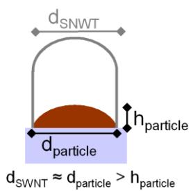
**Supporting Figure S1:** Schematic illustration of the relations of particle height, particle diameter and resulting nanotube diameter.
