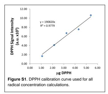
DPPH Calibration of EPR for Quantitative Radical Concentration. 0.0054 g of DPPH was weighed out, placed in a 100 mL volumetric flask, and filled to the line with benzene. From this, 5 different aliquots were pipetted (20, 40, 60, 80, and 100  $\mu$ L), and placed in high purity quartz EPR tubes. The solution was dried by dry nitrogen, and the resulting powder placed under Ar as
