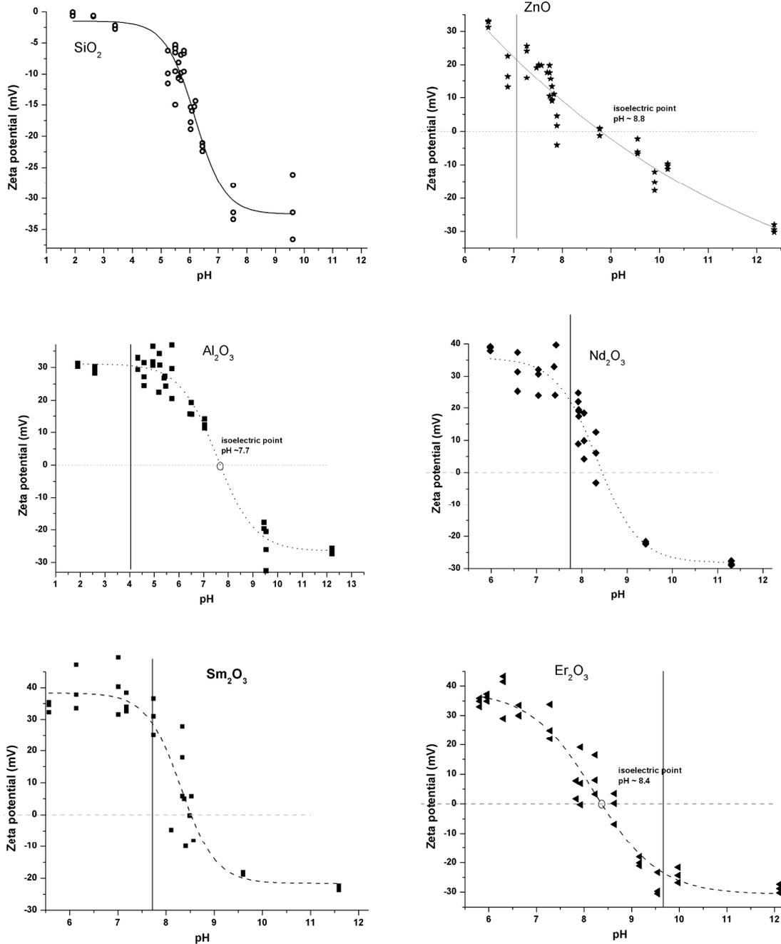
*Zeta potential curves for all studied oxides.* The vertical line indicates the pH of the studied nanoparticle suspensions. Therefore, under our experimental conditions, all nanoparticles are positively charged except SiO<sub>2</sub> and Er<sub>2</sub>O<sub>3</sub>. In the case of silica, the zeta potential is always negative in the studied pH range.
