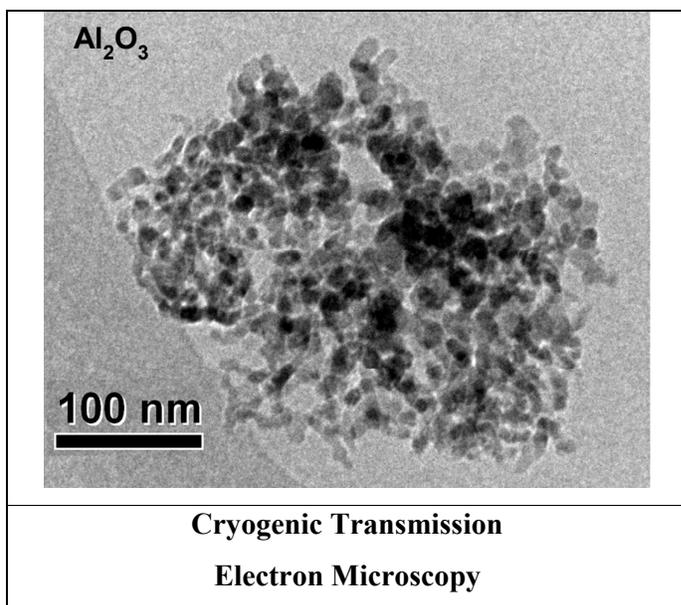
*Cryo-TEM photo of the Al<sub>2</sub>O<sub>3</sub> suspension.*
