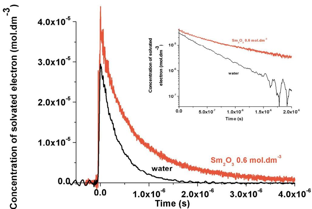
Solvated electron concentration decay recorded after 10-ns electron pulses absorption at 633 nm in a 1 mm optical path cell in water (black) and in an 18% wt (0.6 mol·dm<sup>-3</sup>) Sm<sub>2</sub>O<sub>3</sub> suspension (orange). The two decays are represented with a logarithmic scale in the inset.
