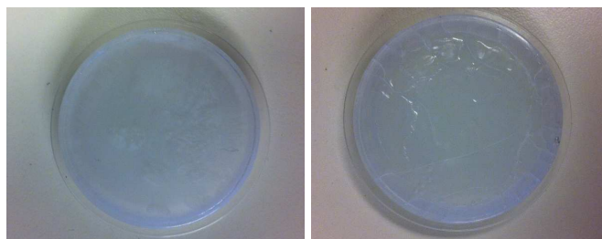
Figure S6. Photograph of bottom (outside) of the PS Petri dish after an sDBF process with a soaking time of 0 min (Left) and 2 min (Right). The Petri dish on the right has been destroyed.
