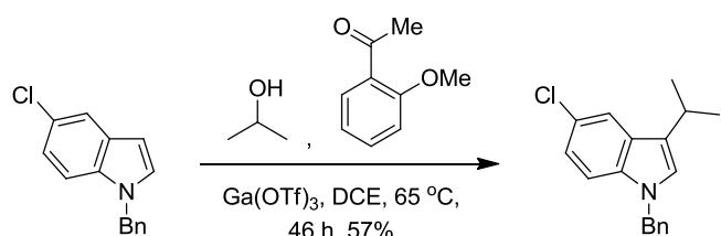
Compound was prepared with modification of a reported procedure.<sup>2</sup> To a mixture of *N*-benzyl-5-chloroindole (1.24 g, 5.1 mmol), 2-methoxyacetophenone (38 mg, 0.26 mmol) and isopropyl alcohol (0.618 g, 10.2 mmol) in dichloroethane (10 mL) was added 131 mg of Ga(OTf)<sub>3</sub>. Reaction was stirred at 65 °C for 46 hours. Solvent was
