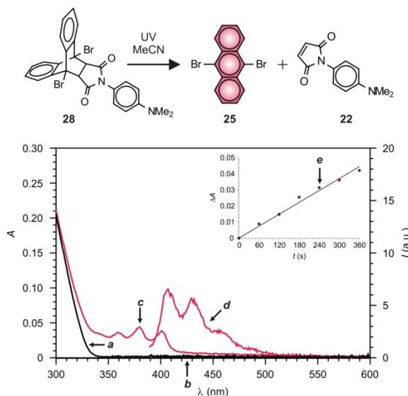
**Figure S16.** Absorption and emission spectra of **28** (40  $\mu$ M, MeCN, 25 °C,  $\lambda_{\text{Ex}} = 370$  nm) before (**a** and **b**) and after (**c** and **d**) ultraviolet (UV) irradiation (254 nm, 0.4 mW  $\text{cm}^{-2}$ , 6 min) and the corresponding absorbance evolution at 380 nm during photolysis.
