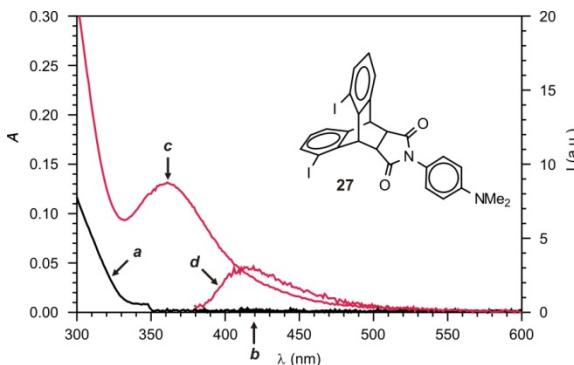
**Figure S15.** Absorption and emission spectra of **27** ( $20 \mu\text{M}$ , MeCN,  $25^\circ\text{C}$ ,  $\lambda_{\text{Ex}} = 370 \text{ nm}$ ) before (**a** and **b**) and after (**c** and **d**) ultraviolet irradiation (254 nm,  $0.4 \text{ mW cm}^{-2}$ , 5 min).
