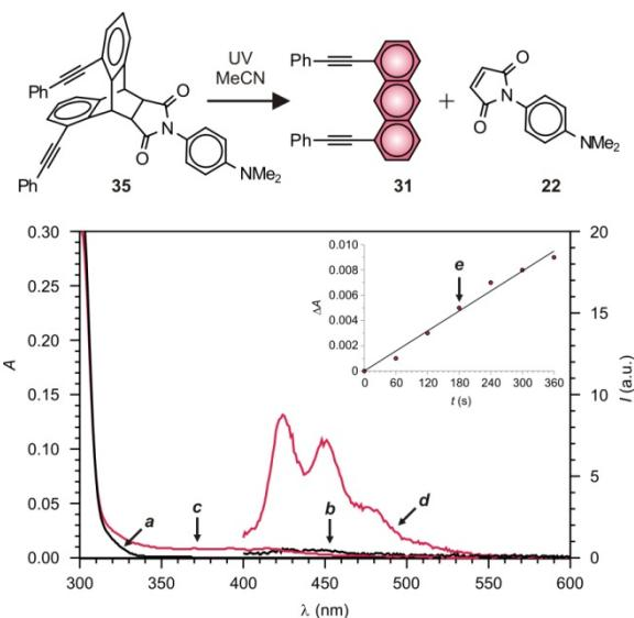
**Figure S18.** Absorption and emission spectra of **35** ( $10 \mu\text{M}$ , MeCN,  $25^\circ\text{C}$ ,  $\lambda_{\text{Ex}} = 390 \text{ nm}$ ) before (**a** and **b**) and after (**c** and **d**) ultraviolet (UV) irradiation ( $254 \text{ nm}$ ,  $0.4 \text{ mW cm}^{-2}$ ,  $6 \text{ min}$ ) and the corresponding absorbance evolution at  $392 \text{ nm}$  during photolysis.
