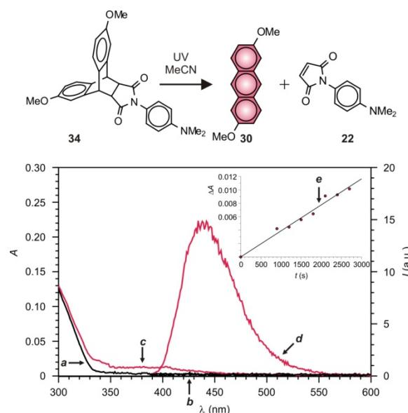
**Figure S17.** Absorption and emission spectra of **34** (30  $\mu$ M, MeCN, 25 °C,  $\lambda_{\text{Ex}} = 350$  nm) before (**a** and **b**) and after (**c** and **d**) ultraviolet (UV) irradiation (254 nm, 0.4 mW  $\text{cm}^{-2}$ , 50 min) and the corresponding absorbance evolution at 401 nm during photolysis.
