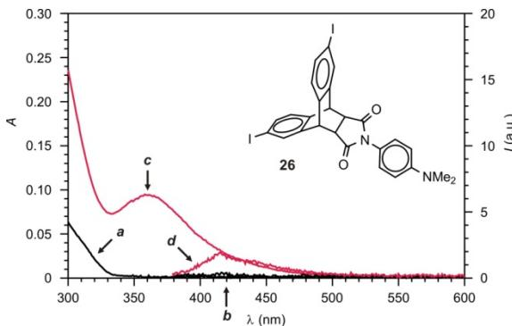
**Figure S14.** Absorption and emission spectra of **26** ( $40 \mu\text{M}$ , MeCN,  $25^\circ\text{C}$ ,  $\lambda_{\text{Ex}} = 373 \text{ nm}$ ) before (**a** and **b**) and after (**c** and **d**) ultraviolet irradiation (254 nm,  $0.4 \text{ mW cm}^{-2}$ , 5 min).
