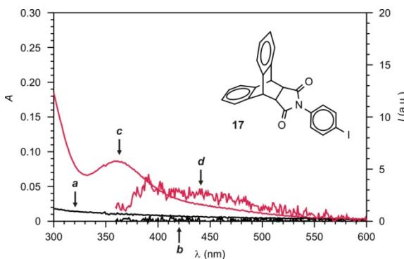
**Figure S13.** Absorption and emission spectra of **17** ( $40 \mu\text{M}$ , MeCN,  $25^\circ\text{C}$ ,  $\lambda_{\text{Ex}} = 350 \text{ nm}$ ) before (**a** and **b**) and after (**c** and **d**) ultraviolet irradiation (254 nm,  $0.4 \text{ mW cm}^{-2}$ , 5 min).
