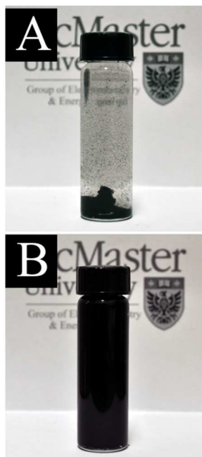
Figure S6. The sedimentation tests for 1 g L -1 of (A) pristine MWCNT and (B) N-AC-MWCNT in 0.5 M Na 2 SO 4 aqueous electrolyte 30 min after ultrasonication.
