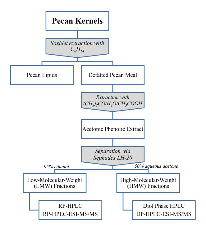
Flow diagram for the preparation of pecan LMW and HMW fractions from a Sephadex LH-20 column and their characterization.
