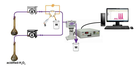
**Figure S2** Schematic diagram of the CL flow-through device.  $P_1$  and  $P_2$ , peristaltic pumps; S, sample injector (carbon dot-DBS-LDHs); F, flow cell; W, waste; PMT, photomultiplier tube (-1100 V);  $H_2O$  at 1.0 mL/min; acidified  $H_2O_2$  at 2.0 mL/min.
