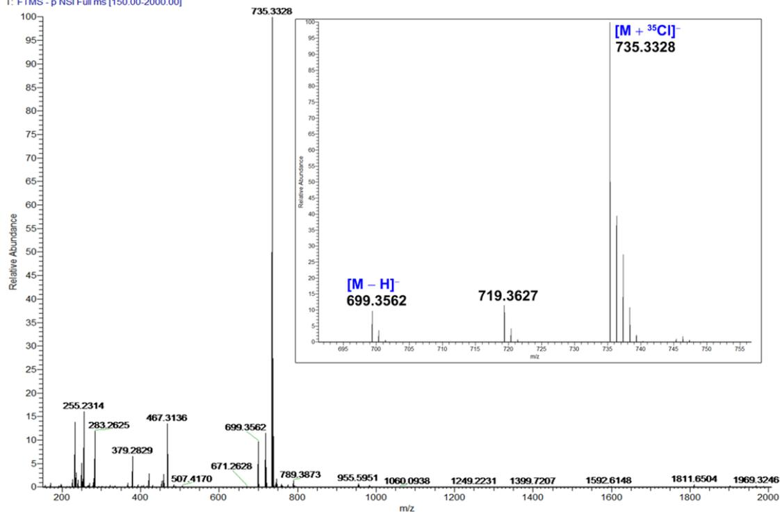
**Figure S1.** HR-ESI-MS (methanol) of host **1** showing adduct formation of  $[1 + \text{Na}]^+$  and  $[1 + ^{35}\text{Cl}]^-$  at highest % abundance in the positive ESI<sup>+</sup> (top) and negative ESI<sup>-</sup> (bottom) respectively.
