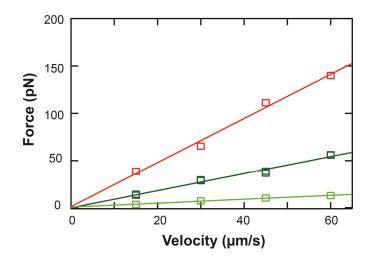
**Figure S1**. Measured deflection as a function of stage velocity near a surface for the three different cantilevers studies, a uncoated long BioLever (*red*), an uncoated BioLever Mini (*dark green*) and a FIB-modified BioLever (*lt green*). The cantilever was moved from in contact to the surface to 100 nm over the surface.
