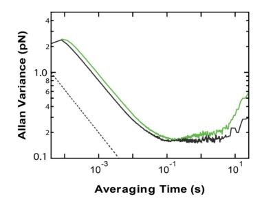
**Figure S3**. Comparing the Allan variance for a FIB-modified cantilever pulling on a surfaceanchored protein [*green* (Figure 6b)] with that of an isolated FIB-modified cantilever [*black* (Figure 3)]. Overall, the sub-pN performance improvements were maintained during a biophysical assay and showed slight worse sub-pN performance at the longest periods. This decrease in performance most likely arises from vertical drift in the commercial AFM.
