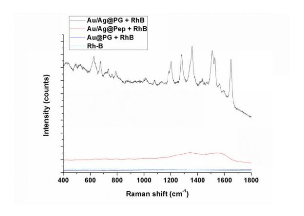
**Figure S8** Raman spectra of surface treated Rhodamin B dye (RhB). RhB was deposited on antibody adsorbed gold chip surfaces additionally covered with Au/Ag@PG (black), Au/Ag@peptide (red), and Au@PG (green). RhB was also deposited on the gold chip without any nanoparticles (blue). Typical Raman peaks of RhB in the 1200~1700 cm<sup>-1</sup> region are 1200, 1282, 1361, 1510, 1533 and 1652 cm<sup>-1</sup>, which agree nicely with above surface-enhanced Raman spectra (Au/Ag@PG + RhB).
