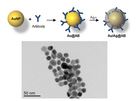
Figure S2 TEM image of silver deposited Au@AB (Au/Ag@AB).
