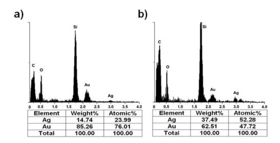
**Figure S3** Single-particle X-ray energy dispersive spectroscopy (EDS) analysis of the prepared Au/Ag core shell nanoparticles, (a) Au/Ag@PG-1 and (b) Au/Ag@PG-2.
