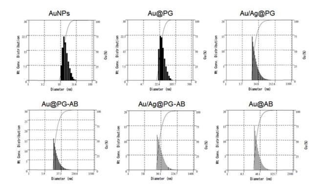
**Figure S5** Direct light scattering (DLS, ELS-Z of Otsuka electronics) measurements: AuNPs ( $d = avg. 14.1 \pm 3.1 \text{ nm}$ ); Au@PG ( $d = avg. 28.3 \pm 8.5 \text{ nm}$ ); Au/Ag@PG ( $d = avg. 29.1 \pm 7.0 \text{ nm}$ ); Au@PG-AB ( $d = avg. 33.4 \pm 7.7 \text{ nm}$ ); Au/Ag@PG-AB ( $d = avg. 34.5 \pm 8.4 \text{ nm}$ ); Au@AB ( $d = avg. 38.3 \pm 19.8 \text{ nm}$ ). Histograms show weight conversion (Wt. Conv.) distributions of the particles.
