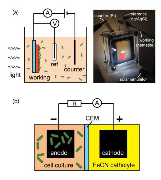
**Figure S1** (a) Scheme and device picture of the solar microbial photoelectrochemical system (solar MPS), configured as a three-electrode photoelectrochemical cell. (b) Scheme of the microbial fuel cell (MFC) device. CEM represents cation exchange membrane.
