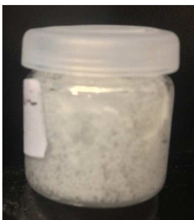
Figure S2 Picture of a vial containing \text{Mg}(\text{BH}_4)_2(\text{NH}_3\text{BH}_3)_2 in argon atmosphere stored at RT for several weeks. The powder has transformed into foam.
