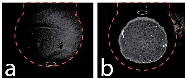
**Figure S5.** Micrographs showing the background fluorescence of the oSlip working electrode (WE) for the Test and (b) Control experiments represented in Figure 3 of the main text. The orange-dashed lines represent the location of the WE. The yellow lines show the areas used to measure the background fluorescence intensity. Note that equivalent areas were used and each experiment was performed in triplicate.
