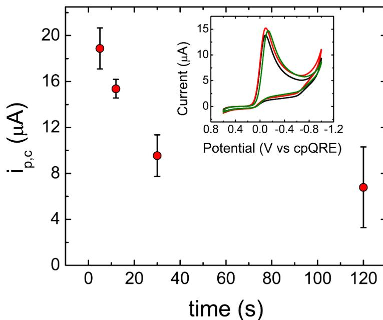
**Figure S9.** Time-dependent study of  $\text{KMnO}_4$  re-solvation in the oSlip. The error bars on each data point represent the standard deviation obtained for three different oSlips. Inset: cyclic voltammograms of  $\text{KMnO}_4$  obtained using three independently fabricated oSlips. The voltammograms were initiated 12 s after slipping Layer 3 into position 2 (Scheme 1c, main text).
