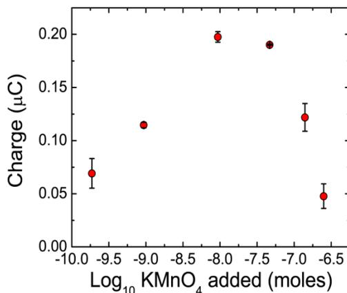
**Figure S7.** Optimization of the electrochemical signal in the conventional electrochemical cell. Plot of charge under the ASV peak as a function of the number of  $\text{KMnO}_4$  moles added. The number of Ag moles was kept constant. The error bars for each data point represent the standard deviation of three different measurements.
