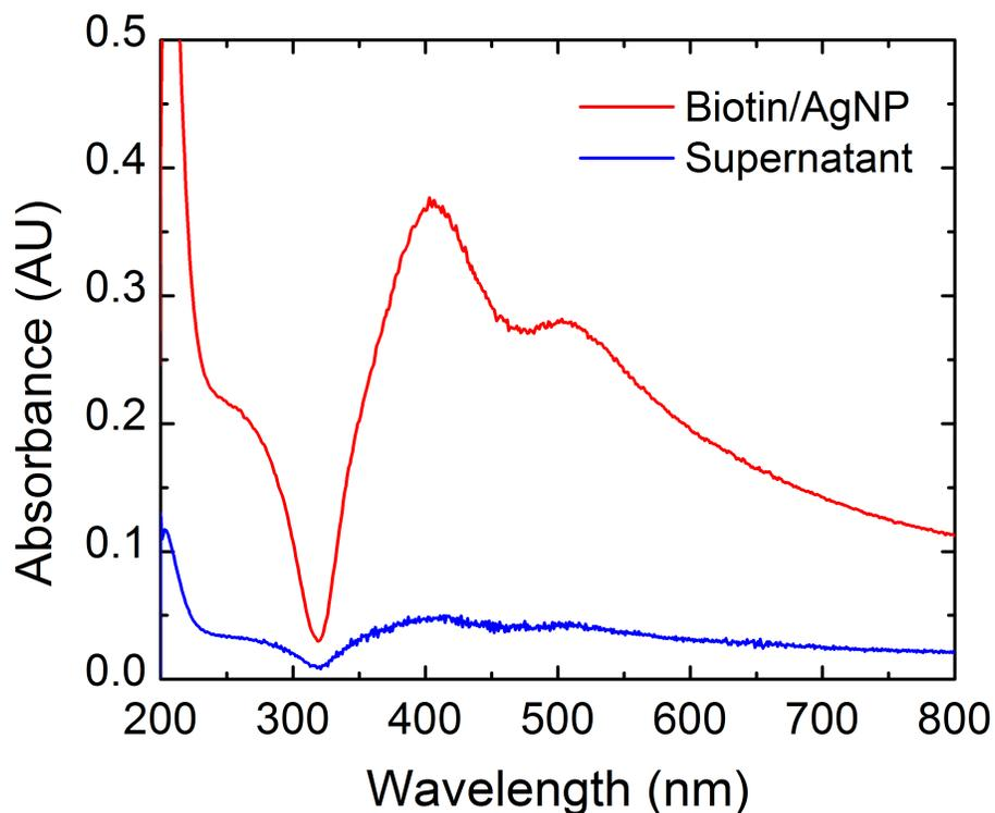
**Figure S6.** UV-Vis spectra showing the formation of the AgNP/biotin/streptavidin/magnetic microbead model analyte. The red trace corresponds to the biotinylated AgNP absorbance before incubation with streptavidin-coated magnetic microbeads. The blue trace corresponds to the supernatant absorbance after incubating biotinylated AgNPs with streptavidin-coated magnetic microbeads.
