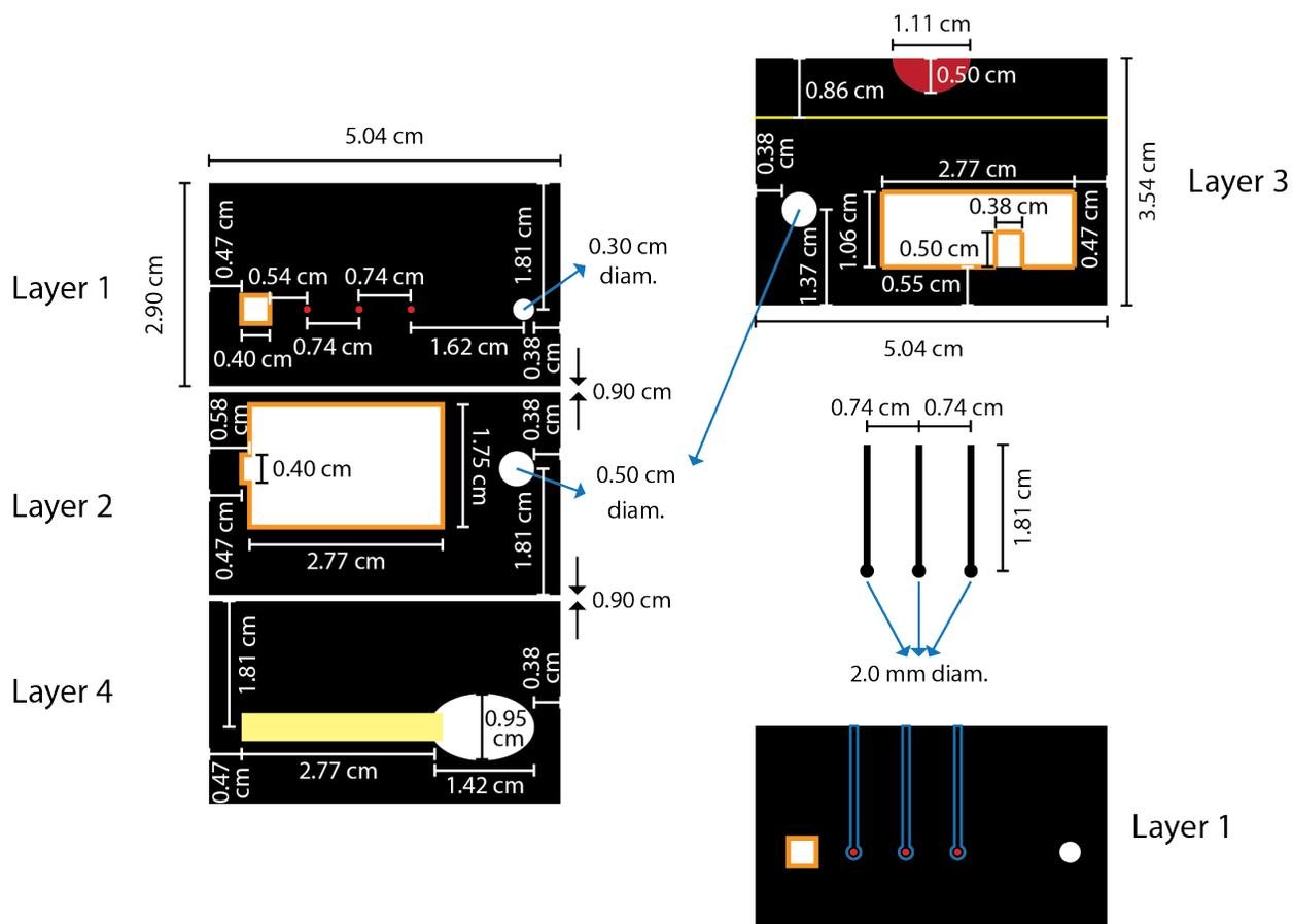
**Figure S2.** oSlip and stencil design and dimensions. *Left:* oPAD portion of the oSlip. *Top right:* SlipPAD portion of the oSlip. *Middle right:* Stencil electrode design. The black areas were cut using a laser engraving system. The width of the rectangular leads is 1.0 mm. *Bottom right:* Position of the stencil on Layer 1. The red dots on Layer 1 serve as a point of reference for alignment. The blue lines represent the outline of the cut stencil.
