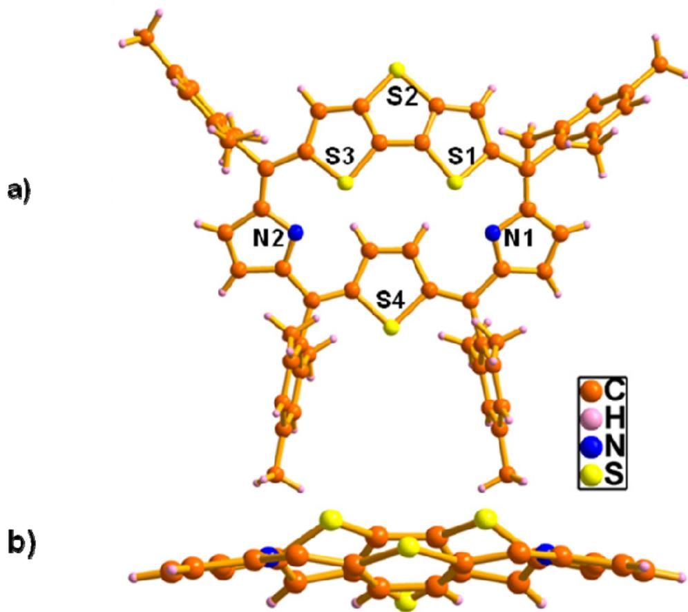
Figure S15. Single crystal X-ray structure of **3** a) Top view b) side view (meso-aryl groups are omitted for clarity)
