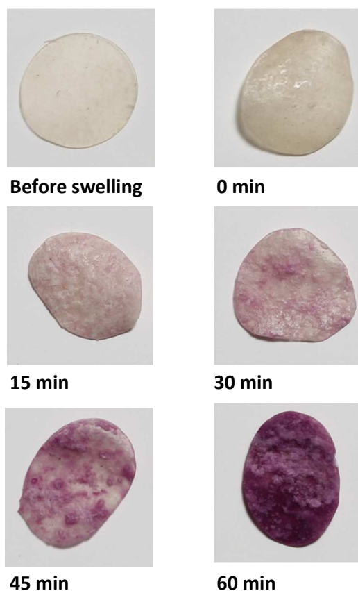
Figure S31. Images of mechanically induced metal exchange in [\text{Eu}(\text{BKB})_{1.5}](\text{ClO}_4)_3 films. Thin films of [\text{Eu}(\text{BKB})_{1.5}](\text{ClO}_4)_3 were swollen in a solution of \text{Fe}(\text{ClO}_4)_2 in \text{CH}_3\text{CN} (10 mL, 0.5 mM) for 5 days. The films were then placed in \text{CH}_3\text{CN} and ultrasonicated for up to 1 h (0.5 sec pulse, 1 sec delay, 20% amplitude). Images of [\text{Eu}(\text{BKB})_{1.5}](\text{ClO}_4)_3 films before and after swelling in an \text{Fe}(\text{ClO}_4)_2 solution, and upon ultrasonication for 15, 30, 45, and 60 min are shown.
