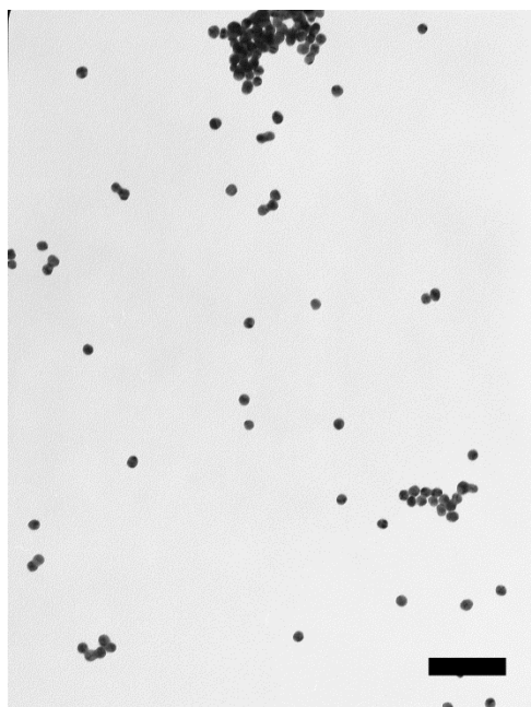
Figure S2. TEM image (scale bar = 100 nm) of 18 nm citrate stabilized gold nanoparticles.
