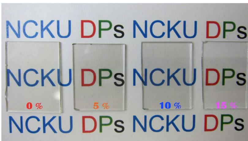
Figure S2. The photos of sputtered NiO<sub>x</sub> films doped with various oxygen flow ratios (0-15 %, from left to right) on ITO-coated substrates.
