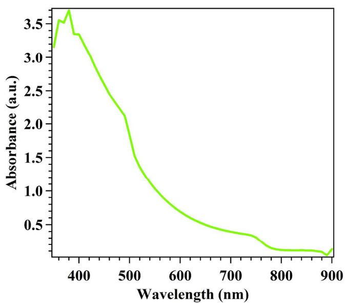
Figure S3. The absorbance of perovskite film coated on mesoscopic NiO nanocrystal layer.
