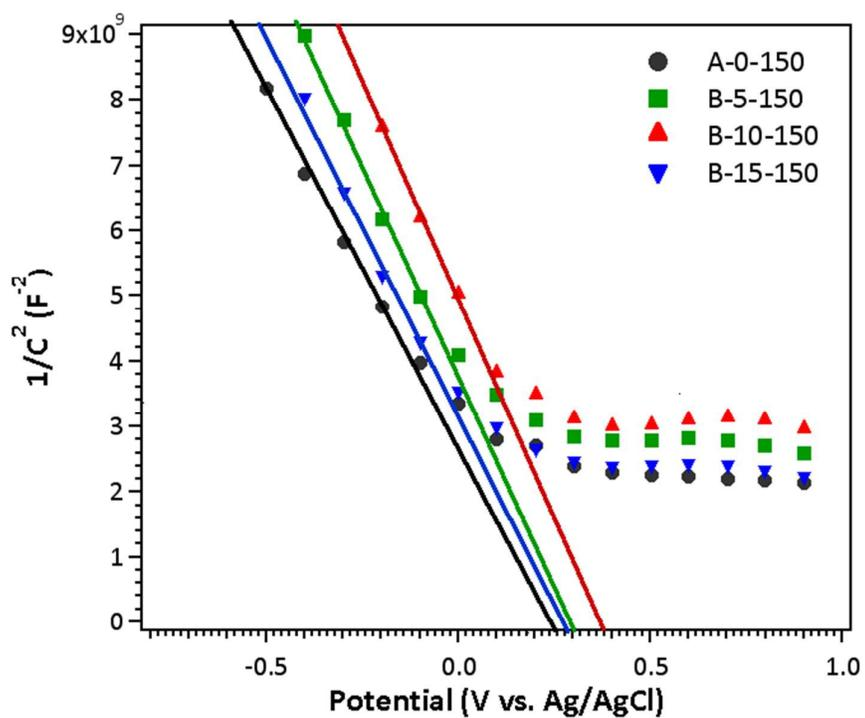
Figure S1. Mott-Schottky plots obtained from sputtered NiOx films doped with various oxygen flow ratios deposited on ITO-coated substrates.
