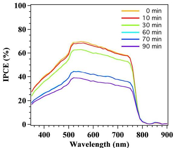
Figure S4. The evolution of IPCE as time during exposure to ambient air without encapsulation.
