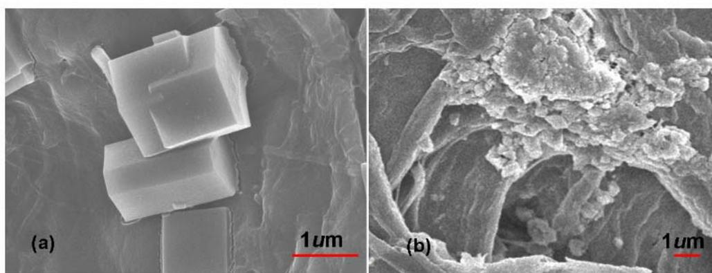
**Figure S4.** (a) Well-shaped crystals of compound **1** were grown in the contact areas of the paper substrate. (b) After breaking crystals by grinding, the samples still can adhere to the surface of paper.
