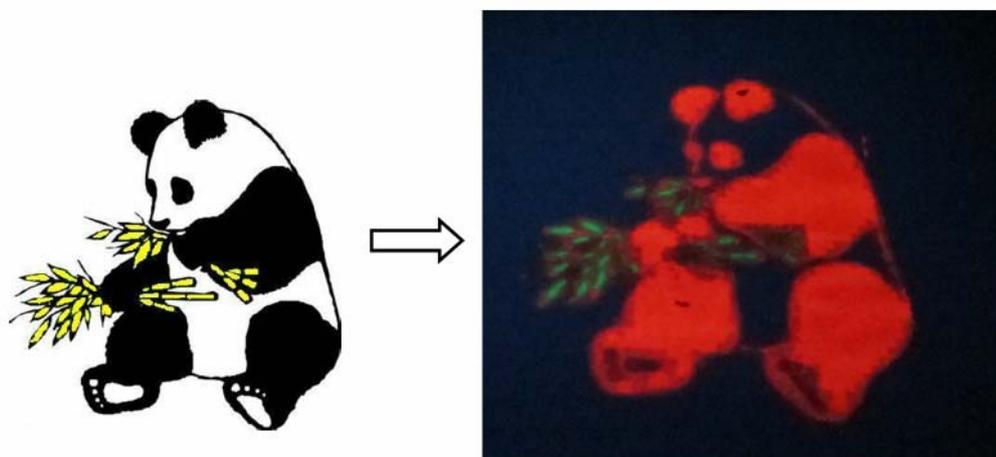
**Figure S6.** Original picture and surface view of a printing sample under illumination of UV light. Red and green emission designated as ‘blank and yellow ink cartridge’ by the Epson coding
