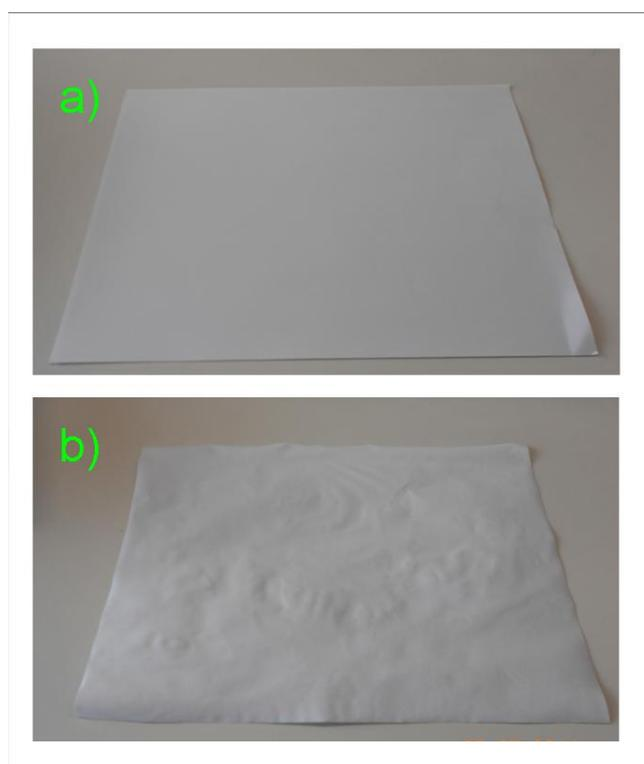
**Figure S3.** Original A4 paper (a) and printed LCCs paper for 8 cycles (b).
