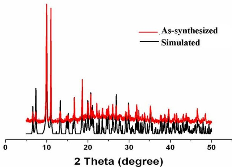
**Figure S1.** XRPD pattern for the as-synthesized sample and the simulated pattern from single-crystal X-ray data of **1**.
