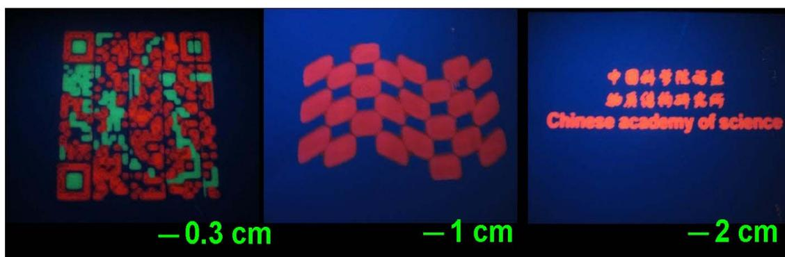
**Figure S7.** Printed LCCs samples with high resolution in varied sizes under excitation of UV light.
