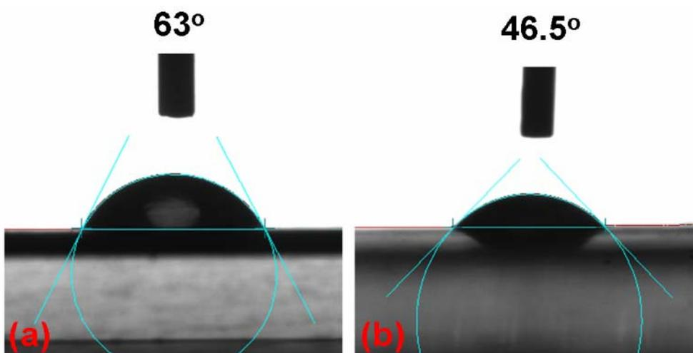
**Figure S5.** (a) Contact angles between the plastic and precursor solution; (b) contact angles between paper substrate and precursor solution.
