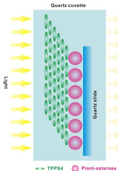
**Figure S4.** Schematic presentation of the spectroscopic measurements using UV-vis absorption, fluorescence, RLS and CD spectroscopies.
