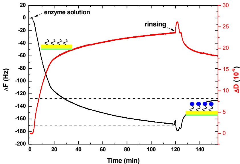
**Figure S3.** All the signal frequency and dissipation variation during plant-esterase immobilization process. It was detected a frequency variation of about -129.7 Hz for plant-esterase immobilization process. From this value and using Voigt model, the mass of plant-esterase immobilized in the self-assembled monolayer of cystamine over the quartz crystal surface was inferred to  $54.27 \text{ mg m}^{-2}$ . The analysis assumed a density of  $1000 \text{ kg m}^{-3}$  for the immobilized layer.
