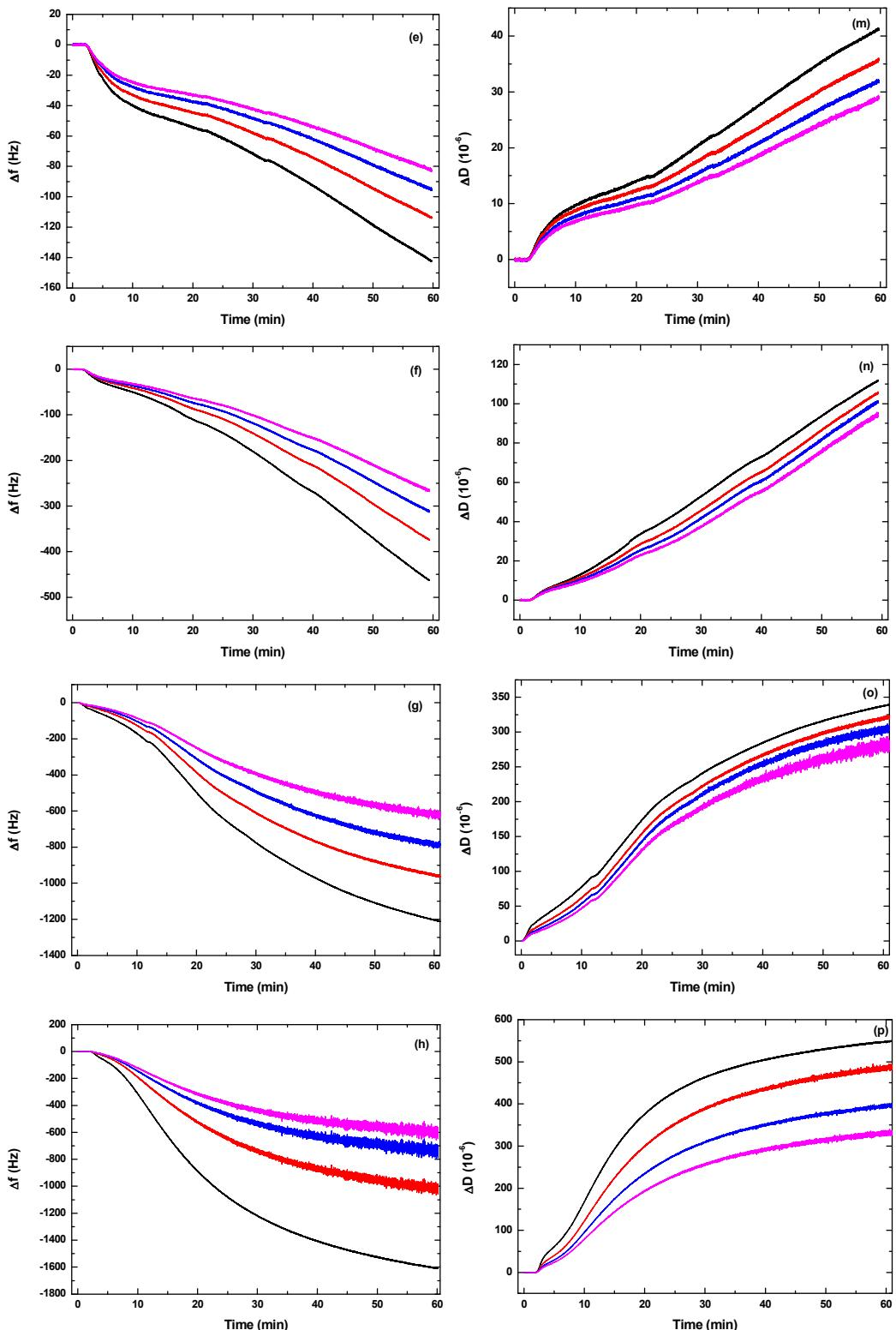
**Figure S5.** Changes in  $f$  (a-h) and  $D$  (i-p) during adsorption of TPPS<sub>4</sub> at eight different concentrations: 0.01 mM (a and i), 0.04 mM (b and j), 0.08 mM (c and k), 0.12 mM (d and l), 0.16 mM (e and m), 0.20 mM (f and n), 0.28 mM (g and o), and 0.36 mM (h and p), at four different frequency overtones: (black) 3rd, (red) 5th, (blue) 7th, and (pink) 9th.
