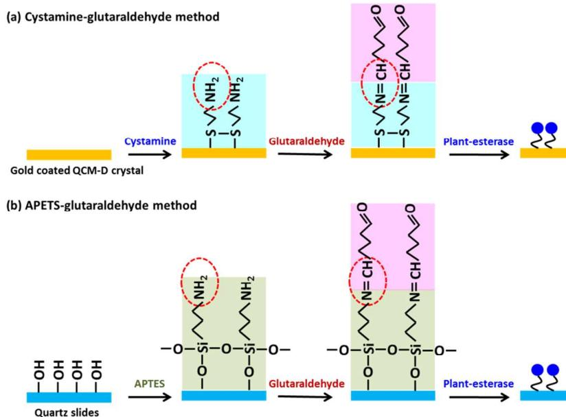
**Figure S2.** The surface modification procedure involved in plant-esterase immobilization on (a) QCM-D gold chip and (b) quartz slides.
