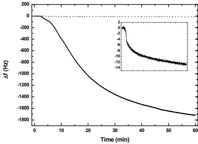
**Figure S6.** Comparison of TPPS<sub>4</sub> adsorption in acidic medium (pH 1.38, line) with that in neutral medium (pH 7.0, points). [TPPS<sub>4</sub>] = 0.44 mM. Inset: expanded view of the points.
