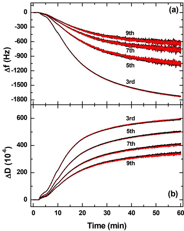
**Figure S7.** Voigt viscoelastic model fitting.  $\Delta f$  (a) and  $\Delta D$  (b) versus time at n=3rd, 5th, 7th and 9th overtones for the TPPS<sub>4</sub> adsorption are shown as black lines. The best fit between the data and the Voigt viscoelastic model is shown as red points. [TPPS<sub>4</sub>] = 0.44 mM.
