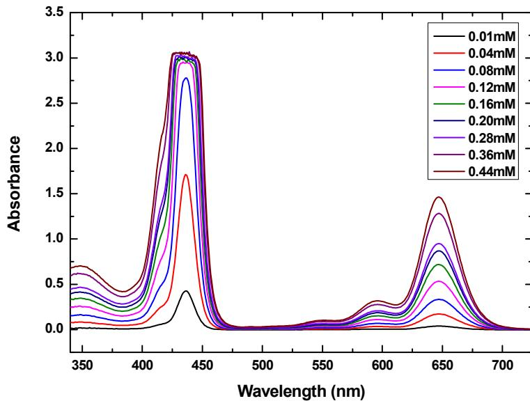
**Figure S1.** Absorption spectra of initial TPPS<sub>4</sub> solutions used for QCM-D measurements. The absorption spectra were collected immediately after the preparation of samples with Shimadzu UV-2450 spectrophotometer using 0.1 cm path length quartz cuvette.
