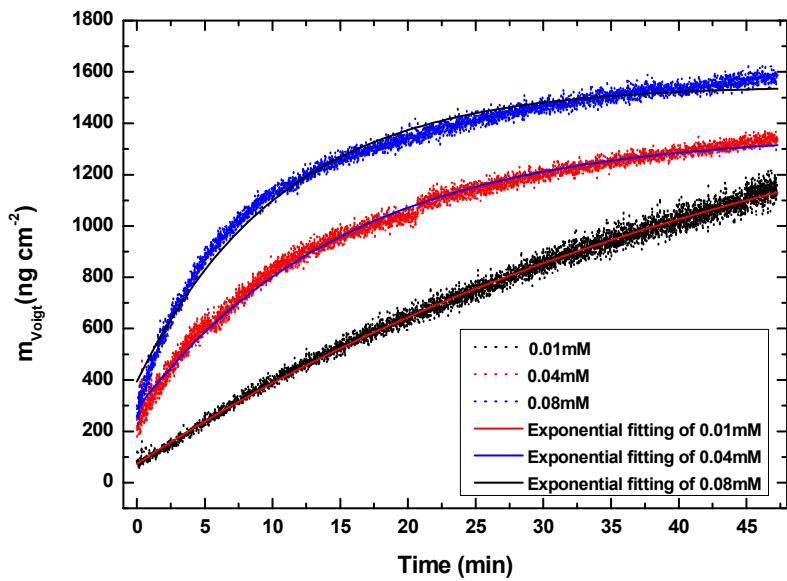
**Figure S8.** Curve fitting for experimental points (dots) and fitted curve for the proposed mathematical equation defining TPPS<sub>4</sub> aggregate nucleation (line).
