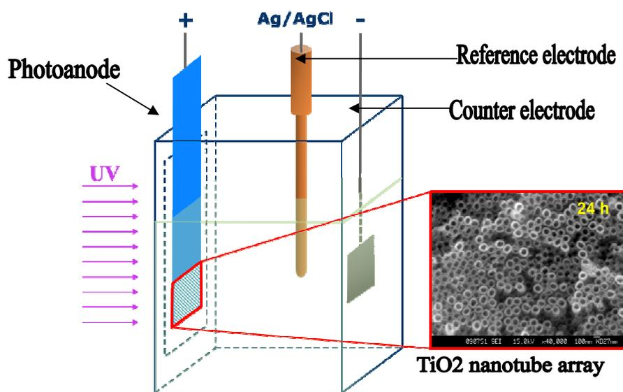
**Figure S1** Schematic diagram of the bulk apparatus for PEC, PC and EC experiments.
