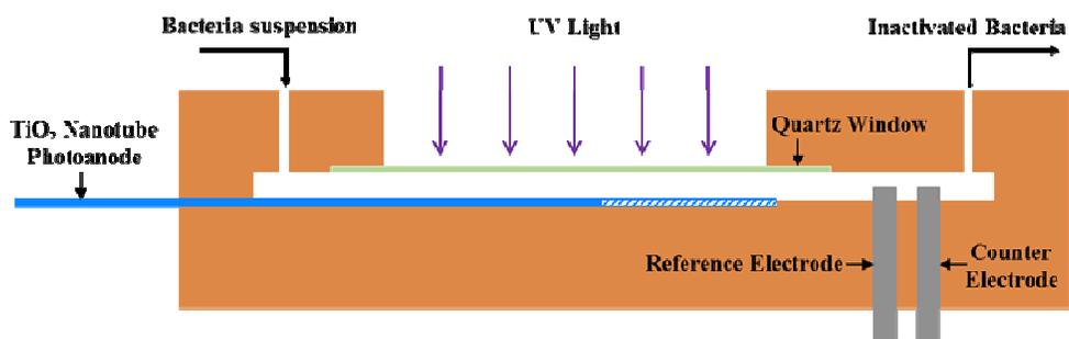
**Figure S4** Schematic diagram of thin-layer reactor.
