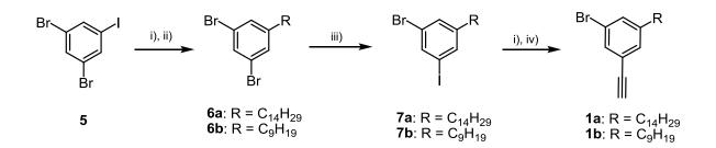
i) Pd(PPh<sub>3</sub>)<sub>2</sub>Cl<sub>2</sub> or Pd(OAc)<sub>2</sub>, PPh<sub>3</sub>, CuI, alkyne, amine, THF; ii) H<sub>2</sub>, PtO<sub>2</sub>, MeOH, toluene; iii) -78 °C, *n*BuLi, I<sub>2</sub>, Et<sub>2</sub>O, THF; iv) K<sub>2</sub>CO<sub>3</sub>, MeOH, CH<sub>2</sub>Cl<sub>2</sub>
