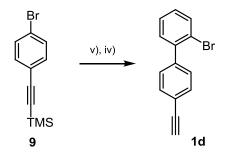
v) *n*-butyl lithium, ZnBr<sub>2</sub>, 2-bromoiodobenzene, Pd(PPh<sub>3</sub>)<sub>4</sub>, Et<sub>2</sub>O, THF; iv) K<sub>2</sub>CO<sub>3</sub>, MeOH, CH<sub>2</sub>Cl<sub>2</sub>
