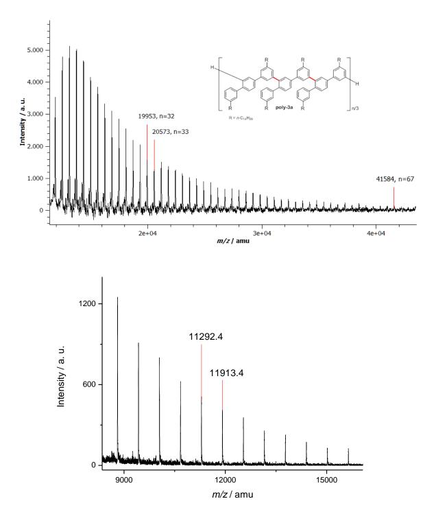
Detail from MALDI-TOF mass spectrum of **poly-3a** recorded with a method selective for lower molecular weights and higher resolution: Only peaks for proton end groups are present in the spectrum; calculated Molecular Weight (n=18+Ag) = 11288.5 g/mol.
