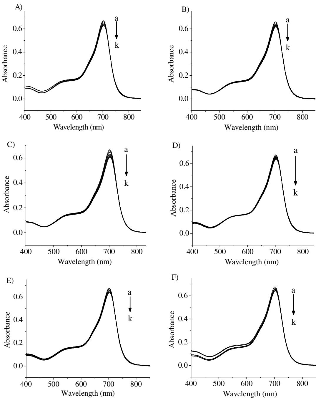
**Figure S9:** Absorption spectral changes showing the negligible interaction of the probe **3a** (12  $\mu\text{M}$ ) with the addition of various competitive anions, a) 0 and k) 40 mM. A)  $\text{SO}_4^{2-}$ , B)  $\text{HSO}_3^-$ , C)  $(\text{S}_2\text{O}_3^{2-})$ , D)  $(\text{NO}_3^-)$ , E)  $(\text{NO}_2^-)$ , F)  $(\text{N}_3^-)$  ions.
