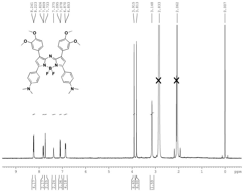
**Figure S3.**  $^1\text{H}$  NMR spectrum of the aza-BODIPY derivative **3c** in Acetone- $d_6$ .
