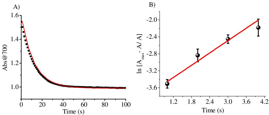
**Figure S7:** A) The temporal profile of absorbance at  $\lambda_{\text{abs}} = 700$  nm observed due to the reaction between probe **3a** and hydrogen sulfide. B) Pseudo first-order kinetic plot of reaction of probe **3a** (5  $\mu\text{M}$ ) with hydrogen sulfide (50  $\mu\text{M}$ ). Slope (Rate constant) =  $0.083 \pm 0.021 \text{ s}^{-1}$ .
