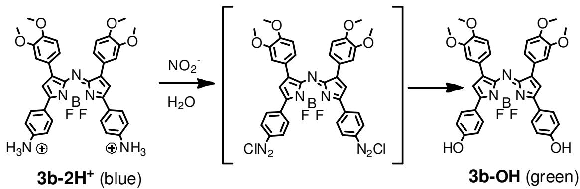
**Figure S10:** Possible mechanism for the detection of nitrite ions sensing using aza-BODIPY derivative **3b**.
