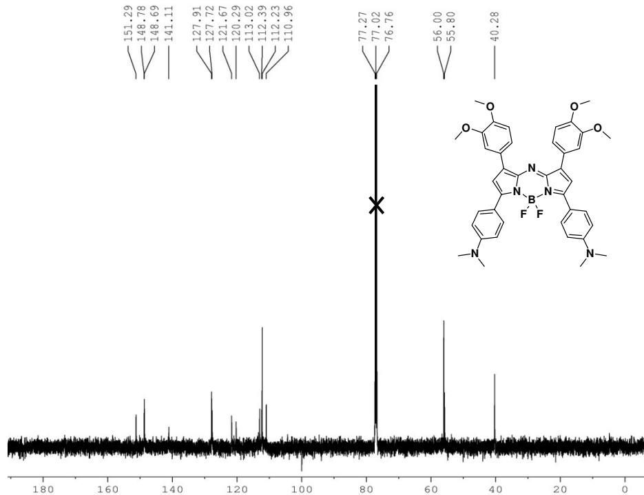
**Figure S6.**  $^{13}\text{C}$  NMR spectrum of the aza-BODIPY derivative **3c** in  $\text{CDCl}_3$ .
