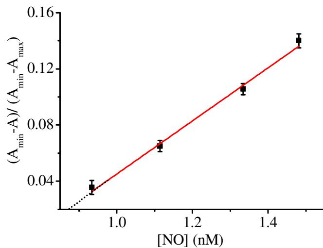
**Figure S11:** Linear plot for the estimation of limit of detection (LOD) from the absorption changes of **3b** with nitric oxide (NO). Data points represent the mean of more than three independent experiments ( $\pm$ SD).
