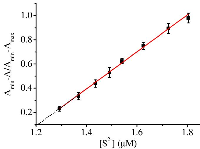
**Figure S8:** Linear plot for the estimation of limit of detection (LOD) from the absorption changes of **3a** with hydrogen sulfide ( $\text{H}_2\text{S}$ ). Data points represent the mean of more than three independent experiments ( $\pm\text{SD}$ ).
