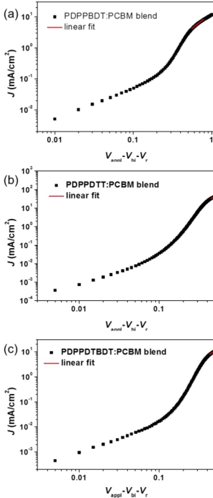
**Figure S5.**  $J$  vs.  $V$  plots for polymer:PC<sub>71</sub>BM blend films. The solid lines are fits of the data points.
