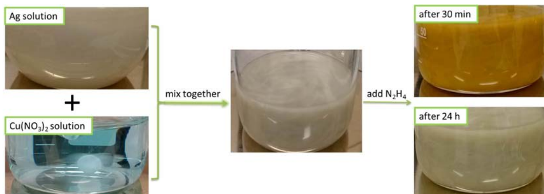
Figure S7. Photographs of reaction systems composited of Ag NWs, Cu (NO 3 ) 2 solution and N 2 H 4 before and after reaction at different stages.
