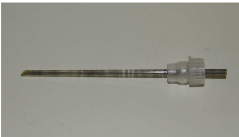
Figure S2. Quartz capillary used for LC-SERS analysis, showing the inside of the tube coated with silver.
