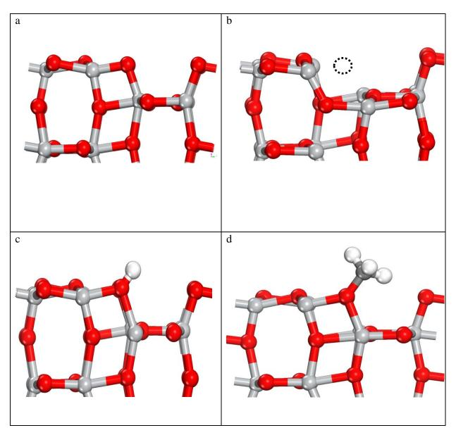
Side views of anatase  $TiO_2$  (100) a) bare surface, b) oxygen vacant surface in plane (missing oxygen is shown as a dotted circle), with c) H adsorbed at the in-planed oxygen, and d)  $\cdot$ CH<sub>3</sub> adsorbed at the in-planed oxygen. Ti is shown in grey (light), O is shown in red (dark), C in dark grey, and H in white.
