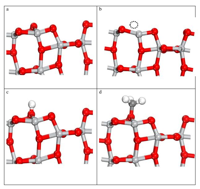
Side views of anatase TiO<sub>2</sub> (101) a) bare surface, b) oxygen vacant surface at the bridge (missing oxygen is shown as a dotted circle), with c) H adsorbed at the bridging oxygen, and d)  $\cdot$ CH<sub>3</sub> adsorbed at the bridging oxygen. Ti is shown in grey (light), O is shown in red (dark), C in dark grey, and H in white.
