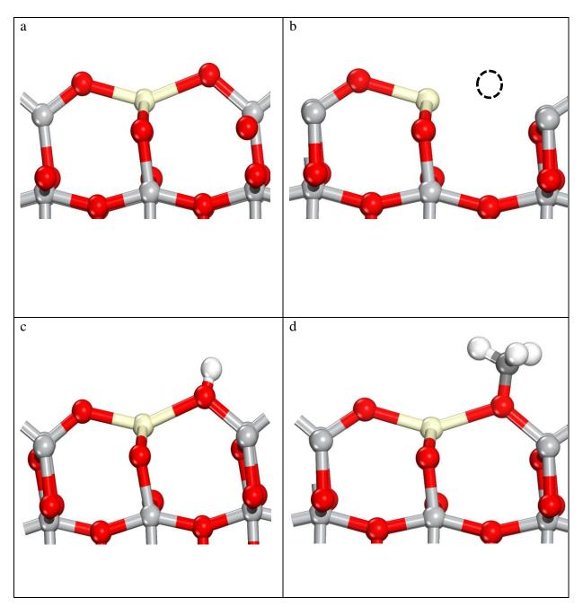
Side views of Ag doped CeO<sub>2</sub> (111) a) bare surface, b) oxygen vacant surface (missing oxygen is shown as a dotted circle), with c) H adsorbed, and d)  $\cdot$ CH<sub>3</sub> adsorbed. Ag is shown in purple (light), Ce is shown in off white (light), O is shown in red (dark), C in dark grey, and H in white.
