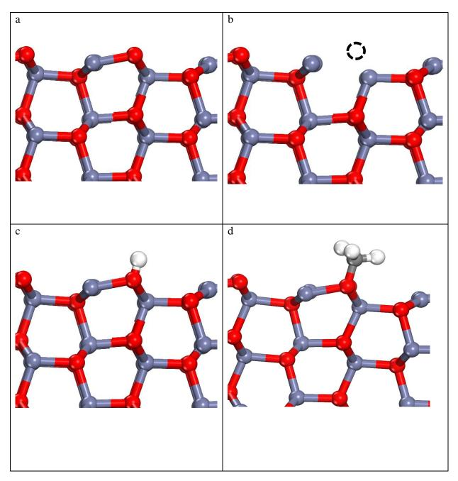
Side views of ZnO (110) a) bare surface, b) oxygen vacant surface (missing oxygen is shown as a dotted circle, with c) H adsorbed, and d)  $\cdot$ CH<sub>3</sub> adsorbed. Zn is shown as grey (light), O is shown in red (dark), C in dark grey, and H in white.
