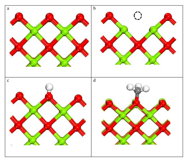
Top view of Pd doped MgO (100) a) bare surface. Side views of Pd doped MgO (100) surface with b) oxygen vacant surface (missing oxygen is shown as a dotted circle), c) H adsorbed, and d)  $\cdot$ CH<sub>3</sub> adsorbed. Pd is shown in blue (grey), Mg is shown in green (light), O is shown in red (dark), C in dark grey, and H in white.
