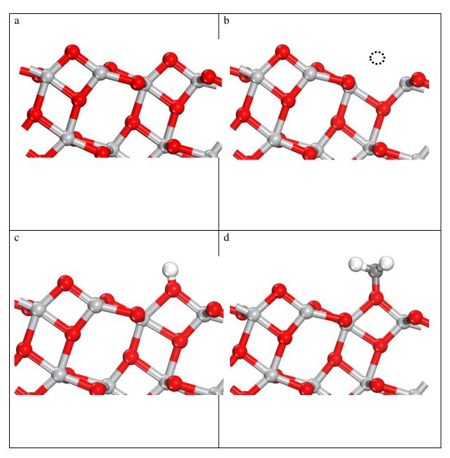
Side views of anatase  $TiO_2$  (101) a) bare surface, b) oxygen vacant surface in the plane (missing oxygen is shown as a dotted circle), with c) H adsorbed at the in-planed oxygen, and d)  $\cdot$ CH<sub>3</sub> adsorbed at the in-planed oxygen. Ti is shown in grey (light), O is shown in red (dark), C in dark grey, and H in white.
