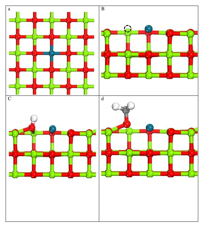
Side views of rutile TiO<sub>2</sub> (110) a) bare surface, b) oxygen vacant surface at the bridge (missing oxygen is shown as a dotted circle), with c) H adsorbed at the bridging oxygen, and d)  $\cdot$ CH<sub>3</sub> adsorbed at the bridging oxygen. Ti is shown in grey (light), O is shown in red (dark), C in dark grey, and H in white.
