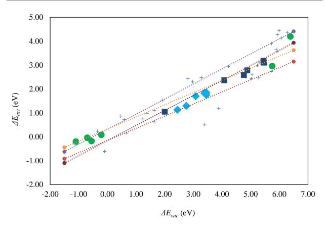
Here, the four dotted lines represent the regression lines with 95% CI coefficients, A and B. All the sub-correlations: varying the U-value for Ce in CeO<sub>2</sub> ( $\diamond$ ), the surface facets for TiO<sub>2</sub> ( $\blacksquare$ ) and the oxidation state for TbO<sub>x</sub> ( $\bullet$ ) lie within this confidence interval.
