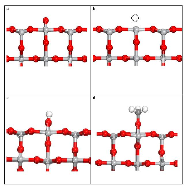
Side views of TbO<sub>2</sub> (111) a) bare surface, b) oxygen vacant surface (missing oxygen is shown as a dotted circle), with c) H adsorbed, and d)  $\cdot$ CH<sub>3</sub> adsorbed. Tb is shown in green (light), O is shown in red (dark), C in dark grey, and H in white.
