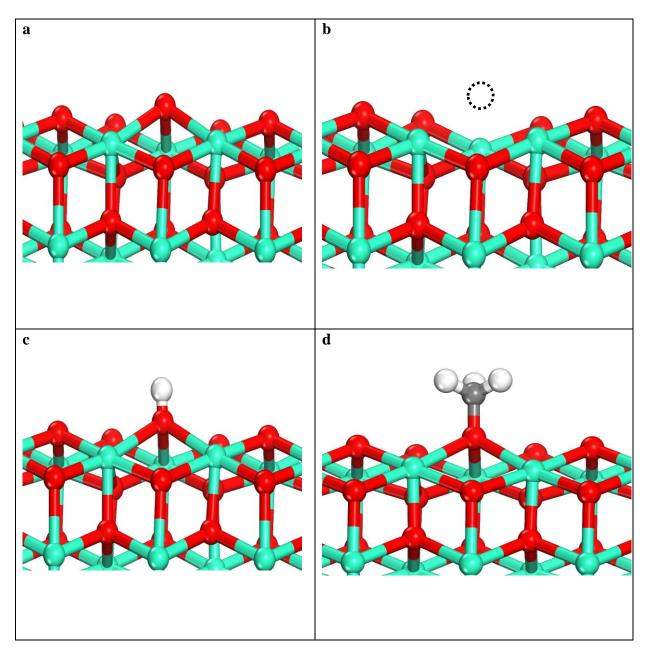
Side views of ZnO (001) a) bare surface, b) oxygen vacant surface (missing oxygen is shown as a dotted circle), with c) H adsorbed, and d)  $\cdot$ CH<sub>3</sub> adsorbed. Zn is shown as grey (light), O is shown in red (dark), C in dark grey, and H in white.
