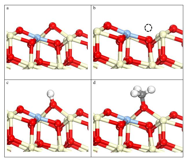
Side views of MgO (110) a) bare surface, b) oxygen vacant surface (missing oxygen is shown as a dotted circle), with c) H adsorbed, and d)  $\cdot$ CH<sub>3</sub> adsorbed. Mg is shown in green (light), O is shown in red (dark), C in dark grey, and H in white.
