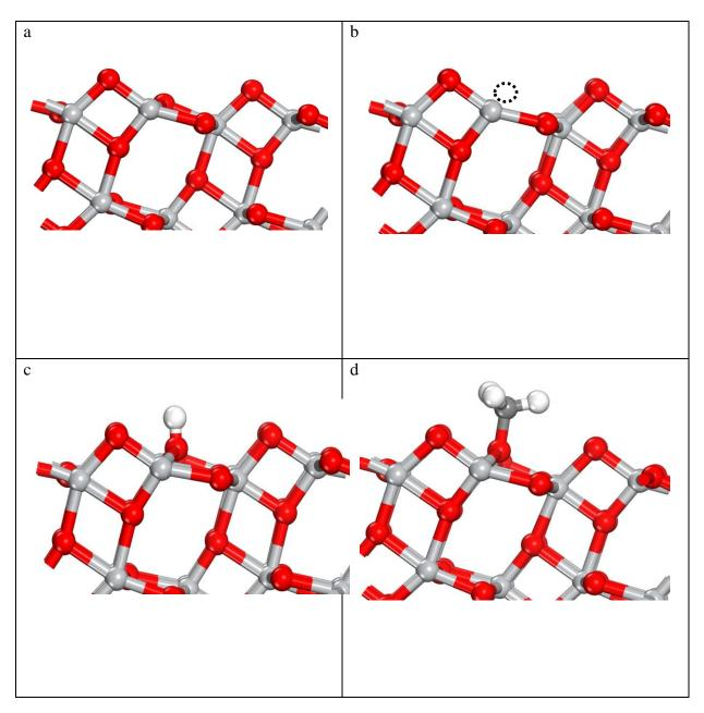
Side views of Ce doped anatase  $TiO_2(001)$  a) bare surface, b) oxygen vacant surface (missing oxygen is shown as a dotted circle), with c) H adsorbed, and d) ·CH<sub>3</sub> adsorbed. Ce is shown in off white (light), Ti is shown in grey (light), O is shown in red (dark), C in dark grey, and H in white.
