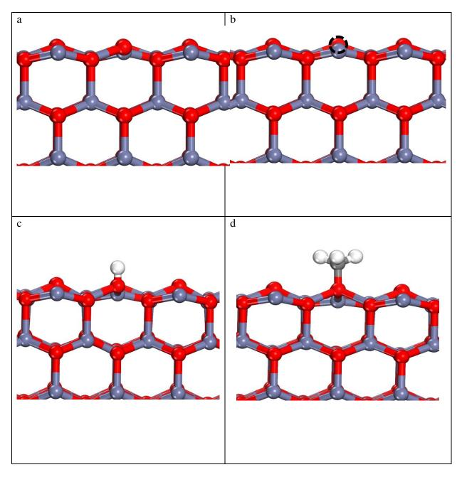
Side views of ZnO (100) a) bare surface, b) oxygen vacant surface (missing oxygen is shown as a dotted circle, with c) H adsorbed, and d)  $\cdot$ CH<sub>3</sub> adsorbed. Zn is shown as grey (light), O is shown in red (dark), C in dark grey, and H in white.
