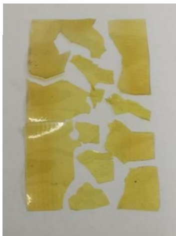
Figure S3. Photographs of (a) F-PAE and (b) ATM-PP after stability test in 0.5 M NaOH at 80°C for 2 h.
