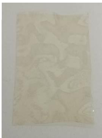
Figure S3. Photographs of (a) F-PAE and (b) ATM-PP after stability test in 0.5 M NaOH at 80°C for 2 h.
