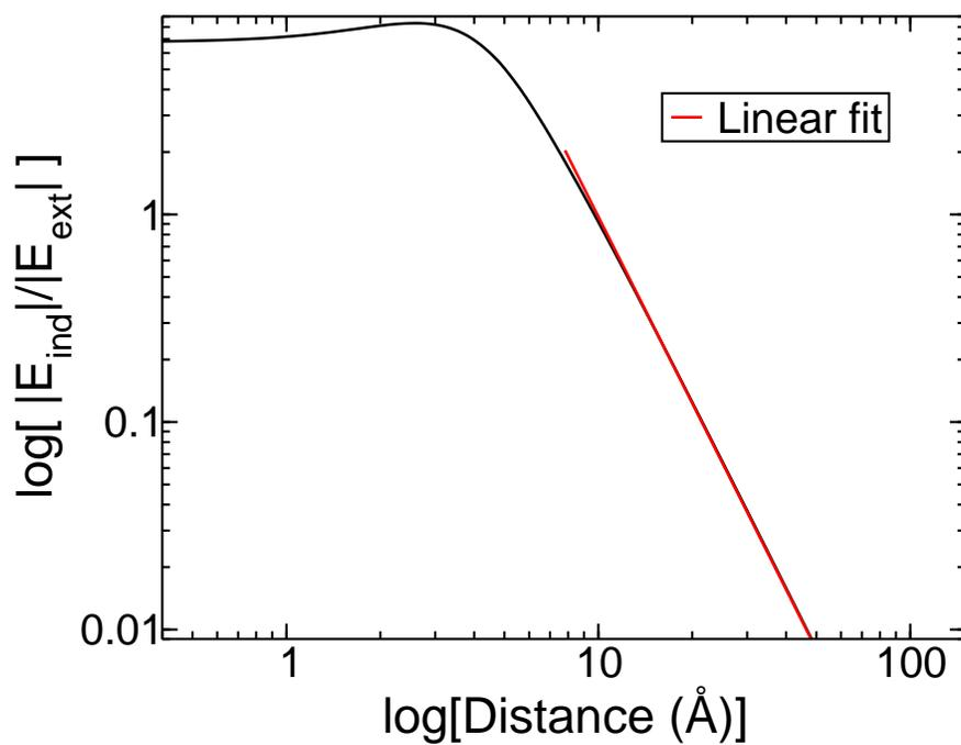
Figure S11: *Log-log plot of the calculated (black line) electric field decay as a function of the distance from the center of the molecule (naphthalene). Red line represents the analytical dipolar behavior  $E_{ind} \propto x^{-3}$ .*
