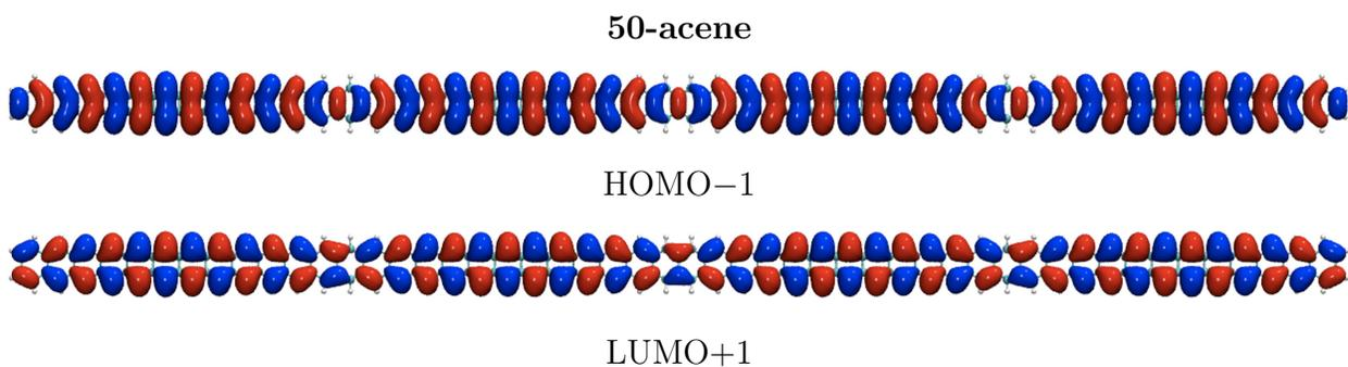
Figure S2: *Isosurface plots of KS HOMO-1 and HOMO+1 molecular orbitals for the 50-acene. Blue and red colors refer to positive and negative values of the orbital wavefunction, respectively.*
