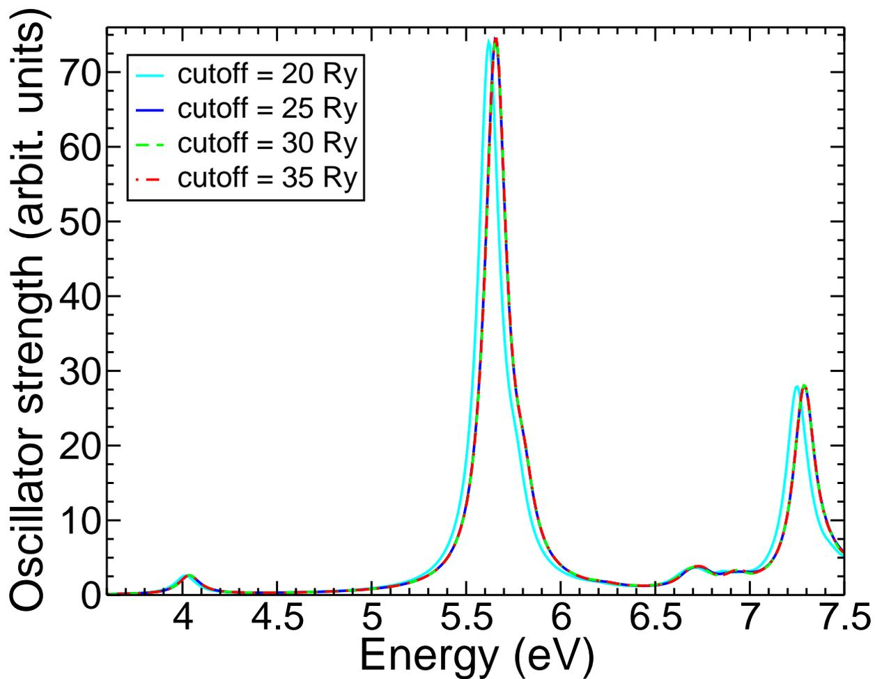
Figure S5: *Low energy absorption spectra of naphthalene: comparison between PBE calculations with different energy cutoffs for the expansion of wavefunctions in plane waves basis set.*
