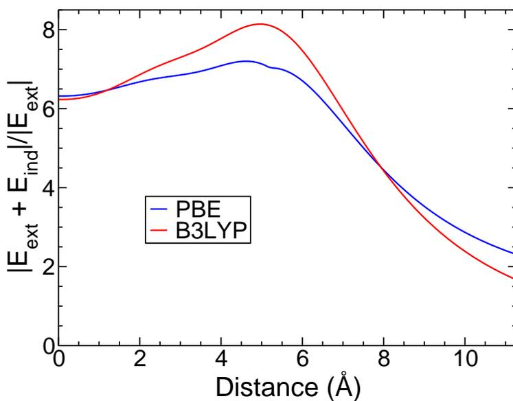
Figure S7: *Electric field enhancement of longitudinally polarized excitations of the tetracene, computed along the axis of the molecule, 3.3 Å above its plane: comparison between PBE and B3LYP calculations. The distance indicated in the x axis refer to the distance from the center of the molecule, on the considered plane.*
