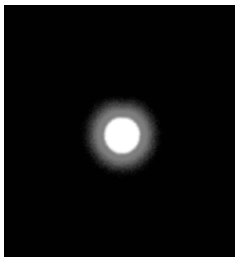
Figure S4. Electron diffraction pattern for homogeneous precipitates in the system containing Fe(III) and arsenate. No diffraction pattern was observed for any system, indicating that all precipitates were amorphous in the early stages of nucleation and growth.
