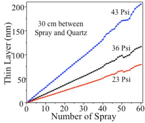
S3. The airbrush-spray deposition setup is shown together with the optimization study of parameters, sample distance and working pressure, for the airbrush-spray.
