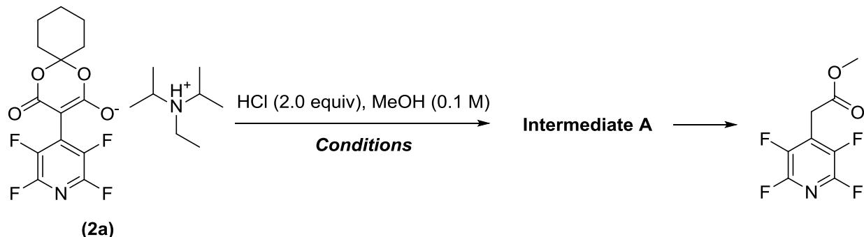
For the monitoring purposes, these reactions were carried out in NMR tubes and monitored via <sup>19</sup>F NMR. Four NMR tubes charged with **2a** (23.1 mg, 0.05 mmol, 1.0 equiv) and HCl (36% w/v, 8.6 μL, 0.1 mmol, 2.0 equiv) and methanol (0.5 mL) were added and sealed glass capillary tubes containing C<sub>6</sub>D<sub>6</sub> were placed in NMR tubes for locking purposes. Then the NMR tubes
