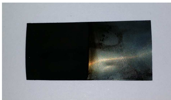
Figure S4. CNF covered on the acid treated (left half) and no CNF observed on the untreated (right half) stainless steel foil.
