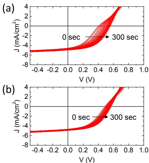
**Figure S1.** Representative  $J$ - $V$  characteristics of inverted P3HT:PCBM BHJ solar cells (ITO/PFN/P3HT:PCBM/MoO<sub>3</sub>/Au) showing reversible degradation after the initial light soaking. (a) The initial light soaking behavior during the first 300 s solar illumination (indicated by an arrow) under AM1.5G, 1 sun solar illumination. (b) Remeasured light soaking behavior of the same device after 12 hr storage under dark condition in vacuum.
