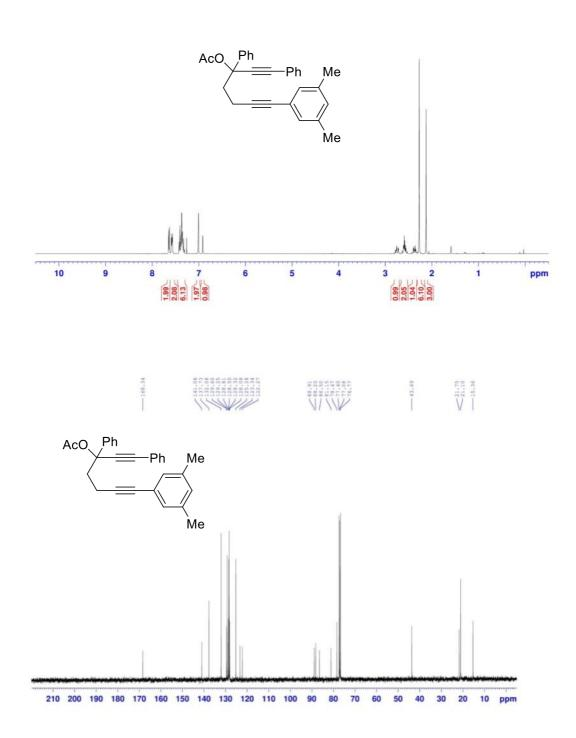
Figure S17. <sup>1</sup>H and <sup>13</sup>C{<sup>1</sup>H} NMR spectra of 7-mesityl-1,3-diphenylhepta-1,6-diyn-3-yl acetate (1q)
