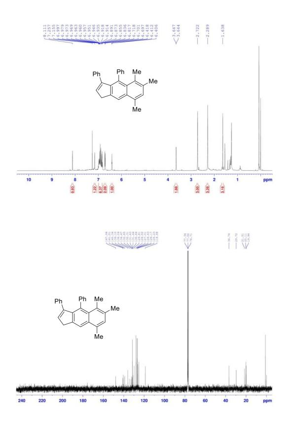
Figure S52. <sup>1</sup>H and <sup>13</sup>C{<sup>1</sup>H} NMR spectra of 7,8-dipho cyclopenta[*b*]phenanthrene (4r)
