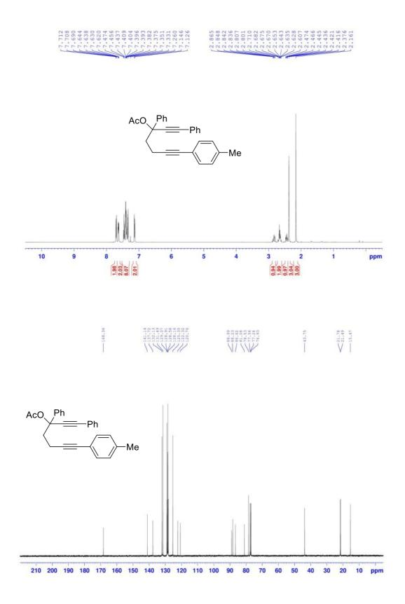
Figure S15. <sup>1</sup>H and <sup>13</sup>C{<sup>1</sup>H} NMR spectra of 1,3-diphenyl-7-o-tolylhepta-1,6-diyn-3-yl acetate (10)
