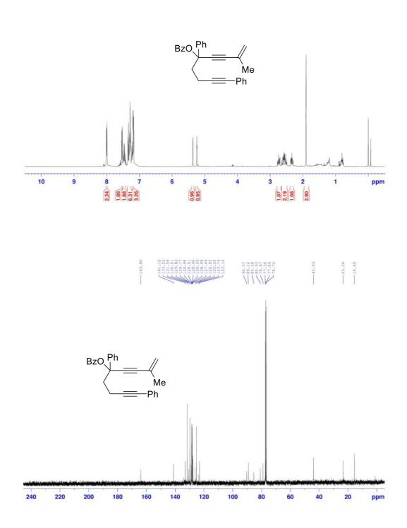
Figure S23. <sup>1</sup>H and <sup>13</sup>C{<sup>1</sup>H} NMR spectra of 2-methyl-5,9-diphenylnona-1-en-3,8-diyn-5-yl pivalate (1w)
