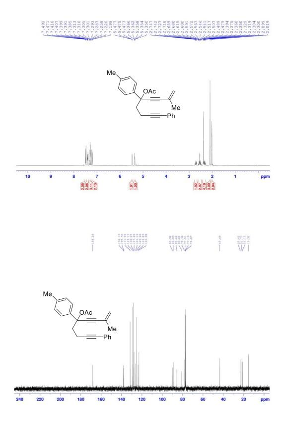
Figure S27. <sup>1</sup>H and <sup>13</sup>C{<sup>1</sup>H} NMR spectra of 2-methyl-5-(naphthalen-1-yl)-9phenylnona-1-en-3,8-diyn-5-yl acetate (1α)
