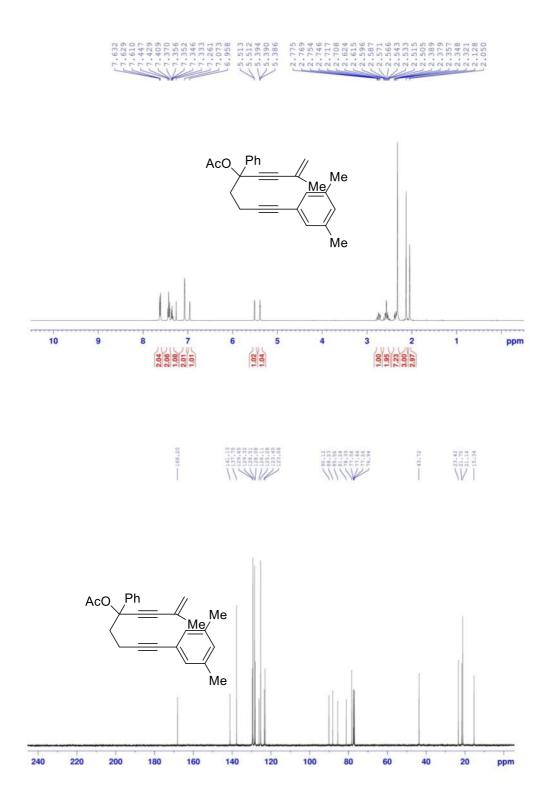
Figure S36. <sup>1</sup>H and <sup>13</sup>C{<sup>1</sup>H} NMR spectra of 2-methyl-5-phenyl-9-(2,4,5trimethylphenyl)nona-1-en-3,8-diyn-5-yl acetate (1κ)
