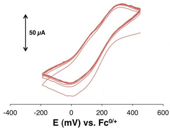
**Figure S19.** Cyclic voltammogram of **4**: 15 scans at 200 mV/s.
