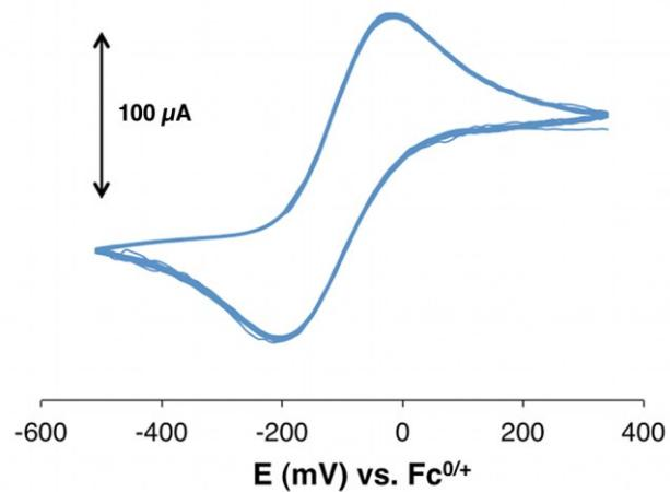
**Figure S16.** Cyclic voltammogram of **3**: 20 scans at 100 mV/s.
