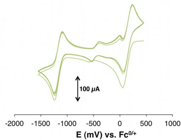
**Figure S22.** Cyclic voltammogram of **5**: 15 scans at 200 mV/s.
