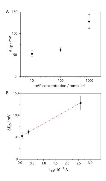
**Figure S8.** Variation of the peak current potential separation  $\Delta E_p$  with: (A) concentration, and (B) peak current measured for three concentrations of pAP [1 mmol L<sup>-1</sup>, 100 µmol L<sup>-1</sup>, 10 µmol L<sup>-1</sup>] in PBS, pH 7.6, at a scan rate of 100 mVs<sup>-1</sup>. In (A), the x-axis is logarithmic.
