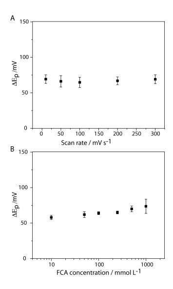
**Figure S7.** Variation of the peak current potential separation  $\Delta E_p = E_{pa} - E_{pc}$  with: (A) scan rate, for a 100 µmol L<sup>-1</sup> solution of FCA in PBS, pH 7.6; (B) concentration of FCA in PBS, pH 7.6, at a scan rate of 100 mV s<sup>-1</sup>. In (B), the x-axis is logarithmic.
