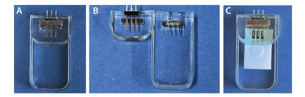
**Figure S4:** PDMS holder (A) consisting of two PDMS parts with embedded magnets (B). The holder can be used to connect the three electrodes (RE, WE and CE) of the electrochemical cell with the cable leads of a potentiostat (C).
