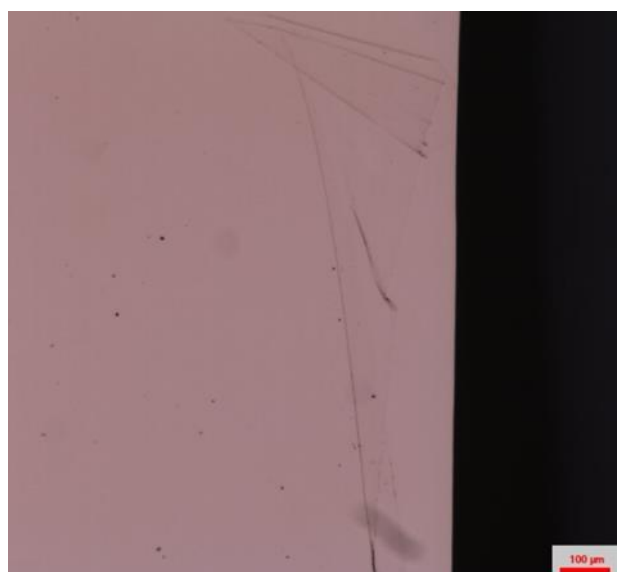
Figure S4: Optical microscope picture from a CMP-membrane after dissolving the SURMOF with EDTA.
